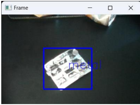
Figure 11.1.: The model can detect shining metal surfaces quite well.
