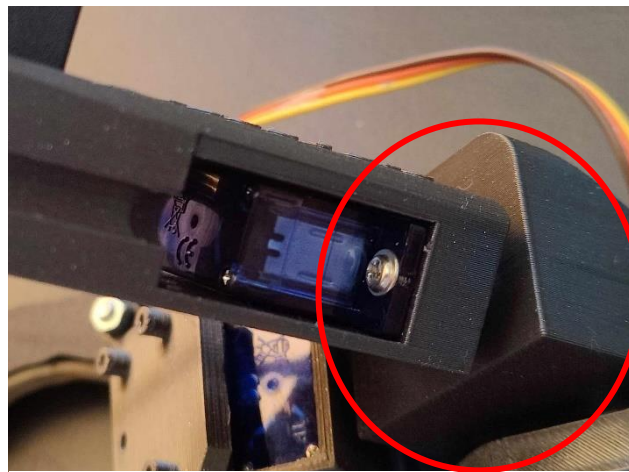
Figure A4.: An SG90 servo screwed inside the second arm part with the help of two servo screws, on the tip of that came the third arm part [highlighted]
