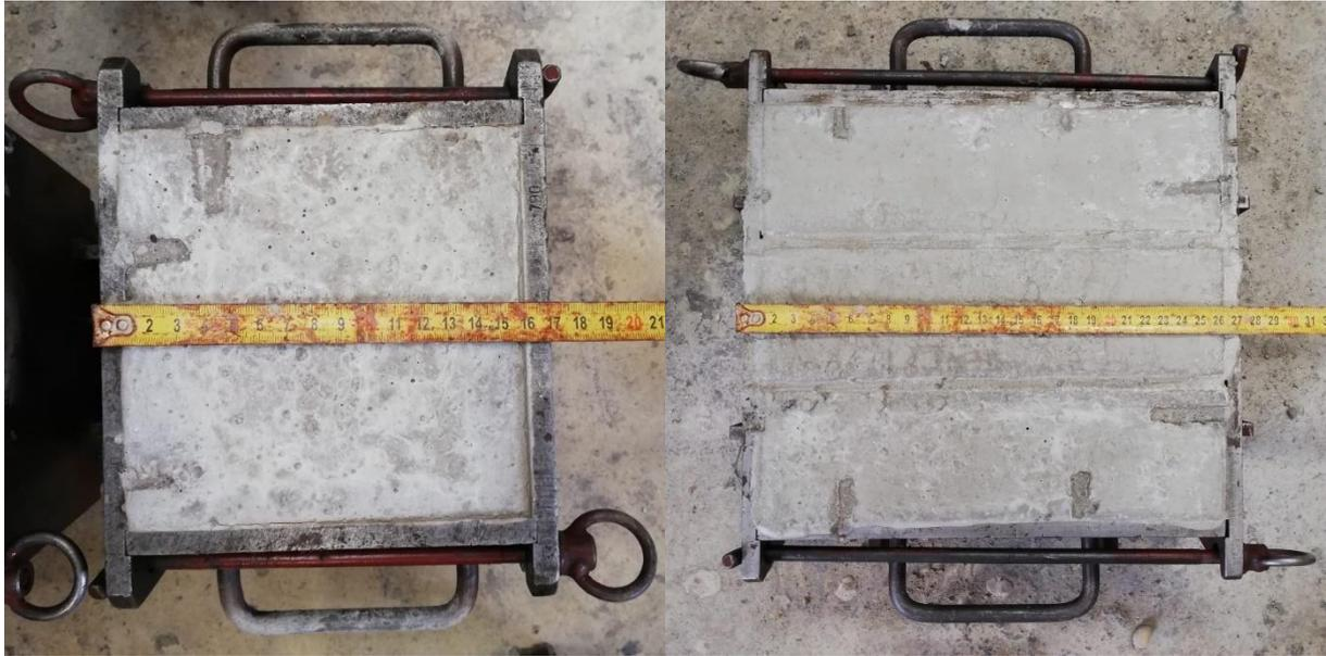
**13. Figure** *Mould for a cube specimen (left) and prism specimens (right)*
