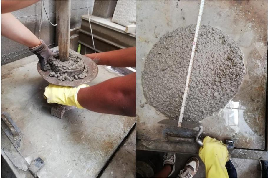
**11. Figure** *Consistency measurement on the flow table*
