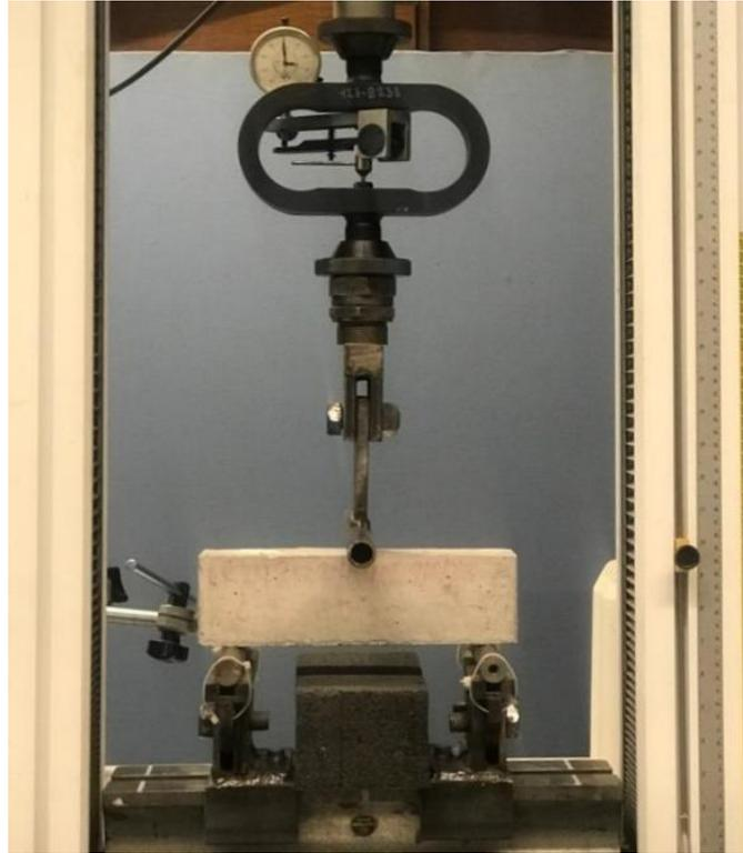
**16. Figure** *Flexural tensile test on prisms*
