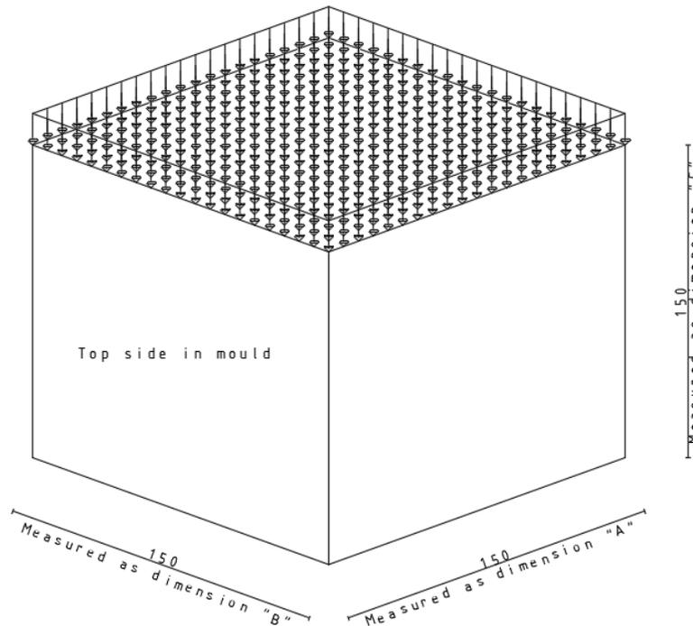
**15. Figure** *Schematic representation of the compressive strength measurement, with average dimensions in millimetres (made with the AutoCAD software)*
