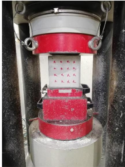
**14. Figure** *Compressive strength measurement on cubes*
