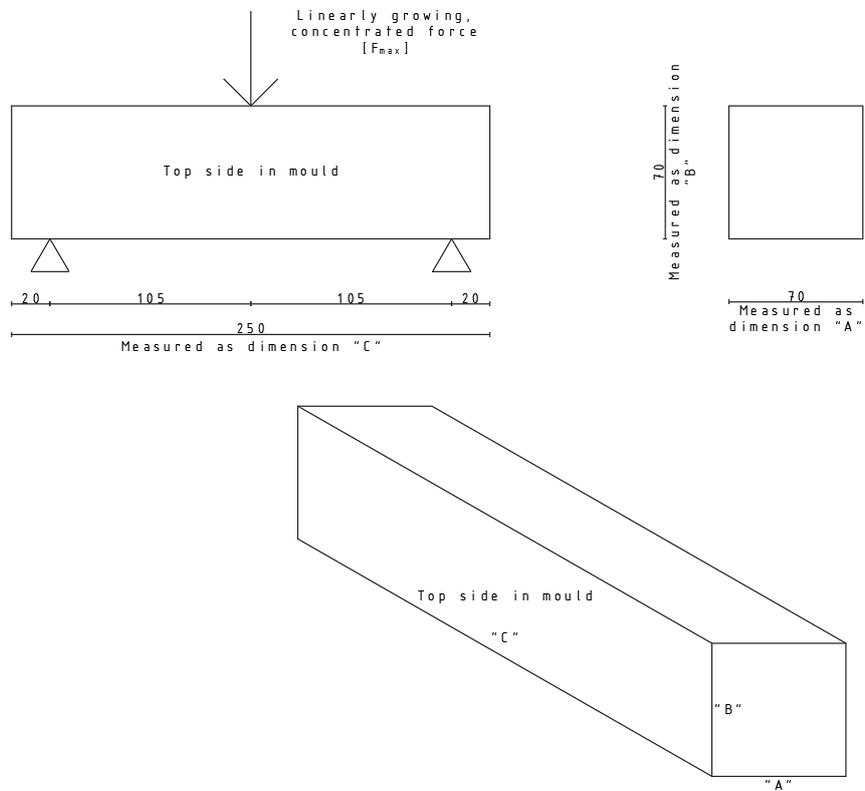
**17. Figure** *Schematic representation of the flexural tensile strength measurement, with average dimensions in millimetres (made with the AutoCAD software)*
