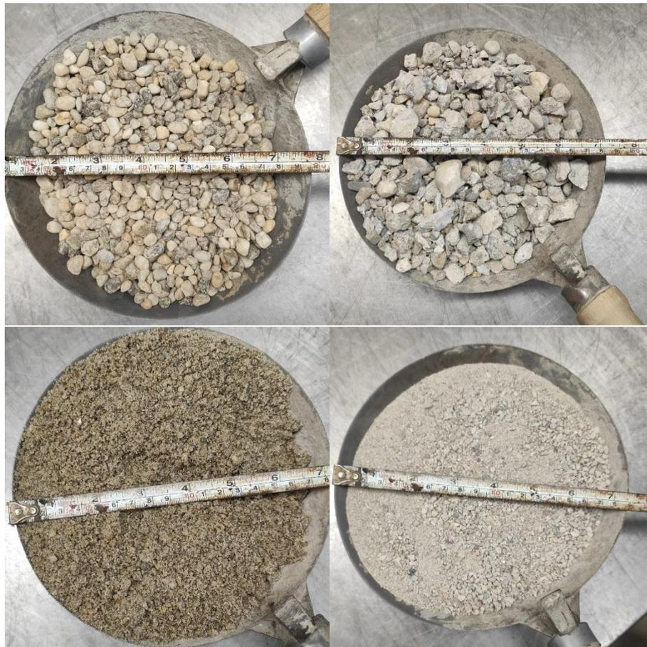
**9. Figure** *The aggregates of the experimental concrete. Clockwise, from top left to bottom left: coarse natural aggregate, coarse recycled aggregate, fine recycled aggregate and fine natural aggregate*
