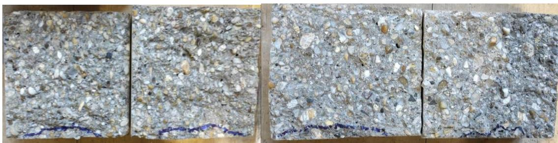
*Highlighted water penetration marks on the specimen [Figure 9]*
