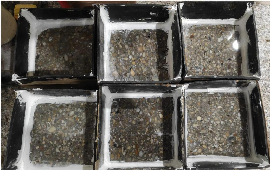
*Specimens covered with rubber sheets and 3mm of water added on top [Figure 11]*
