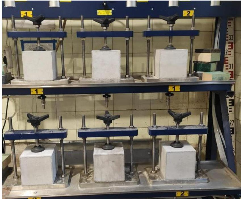
*Specimens placed in water tightness apparatus [ Figure 8]*
