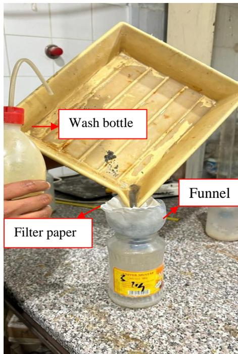
*Collection of the scaled material using a funnel, filter paper and wash bottle [Figure 13]*
