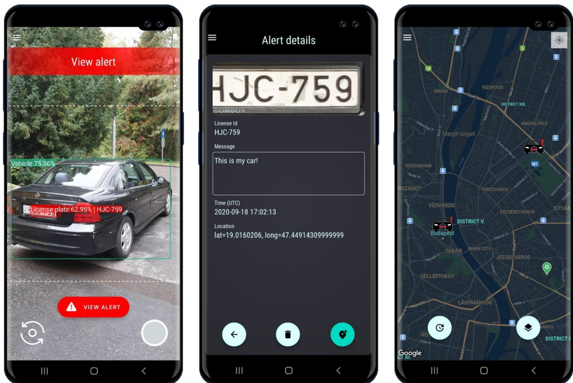
Figure 31: Live inference (left), recognition details (middle), map of detected vehicles (right)
