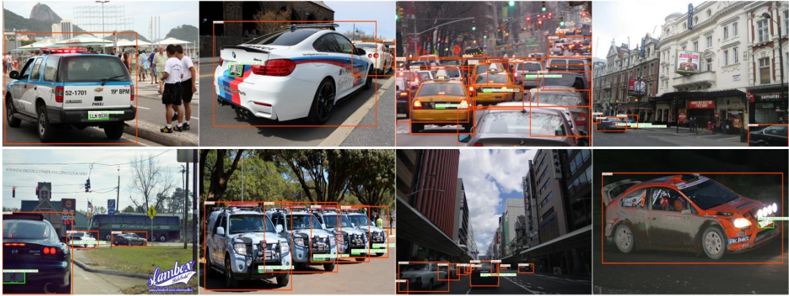
Figure 10: Validation (1 st row) and test (2 nd row) samples with boxes (vehicle reg. plate, vehicle)
