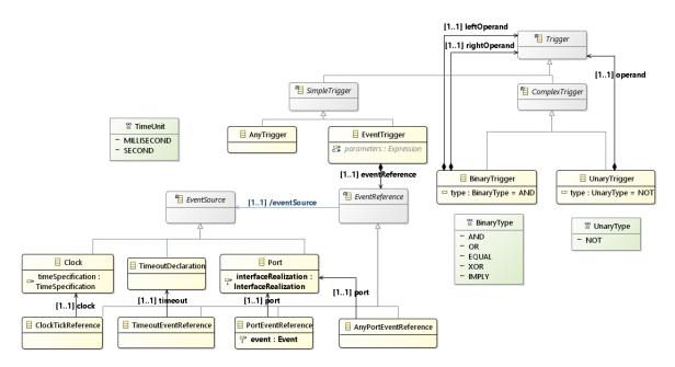
Figure 3.5: The part of the gamma metamodel supporting the definition of triggers.
