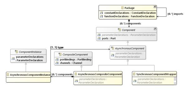
**Figure 4.4:** Fragment of the metamodel describing the asynchronous component types.
