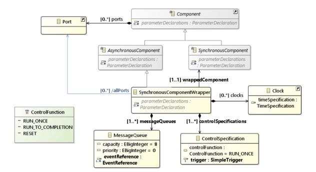
Figure 4.5: Fragment of the metamodel describing the synchronous component wrapper element.
