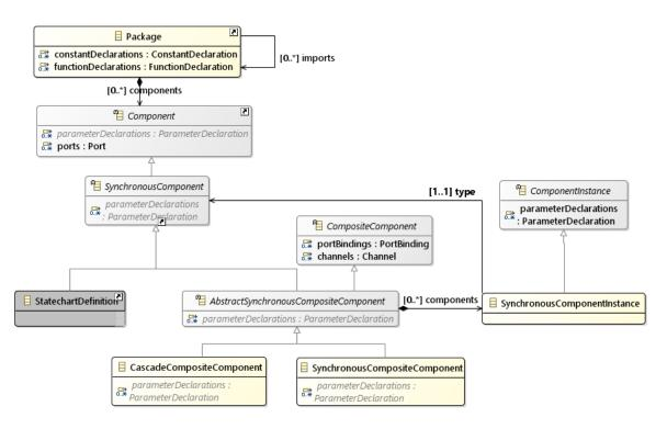
Figure 4.3: Fragment of the metamodel describing the synchronous component types.
