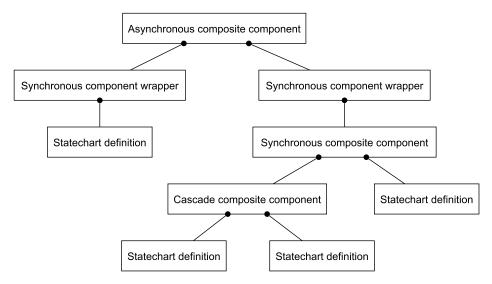
Figure 4.6: A composite model hierarchy in gamma.
