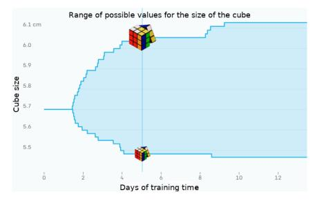
Figure 2.6: Automatic Domain Randomization automatically widens the randomization parameters during training (modified figure of [29]).
