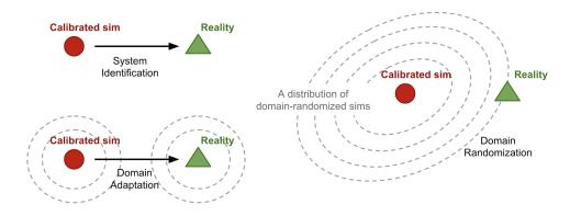
Figure 2.3: Overview of the approaches of sim-to-real transformation (source: [19]).
