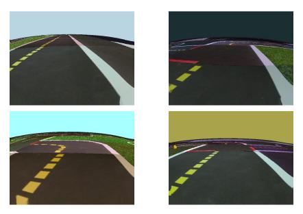
Figure 3.2: During training, the visual parameters, such as colors and textures, of the simulation environment are randomized.
