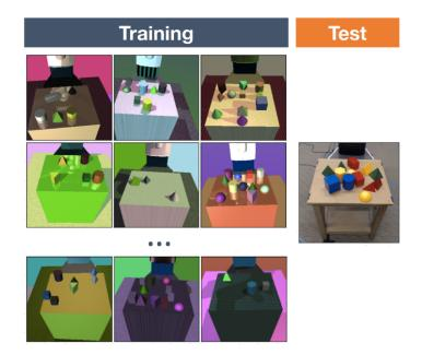
Figure 2.5: Illustration of domain randomization for robotic grasping (source: [27]).
