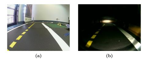
Figure 5.4: Camera images from the robot in daytime (a) and night (b) visual conditions. The agent was taught in the simulator only in daytime visual conditions, but it is able to drive in night visual conditions as well.
