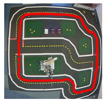
Figure 5.3: The path of the agent in the real-world environment. The picture was created by recording a video with a camera placed above the track and using the CSR-DCF object tracking algorithm [38]. Due to the camera not being completely above the track, the image has distortion on its right side, and the path is not displayed accurately here.
