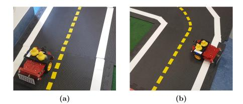
Figure 5.5: Extreme test cases include starting the vehicle from invalid locations: the oncoming lane (a) and cross the road (b). My experiments showed that the agent is able to recover from these starting positions to the right lane and continue driving there.
