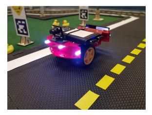
Figure 4.2: Duckiebots are small three-wheeled robots with a forward-facing camera. It has to be controlled by processing the camera images and giving wheel speed commands.
