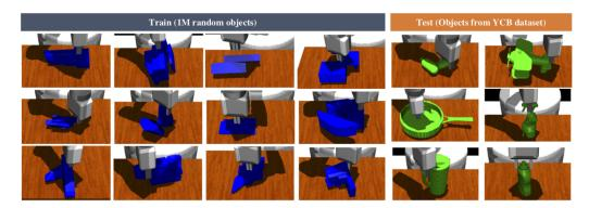
Figure 2.7: Training a model on lots of procedurally generated objects makes it able to generalize to realworld objects as well (source: [30]).
