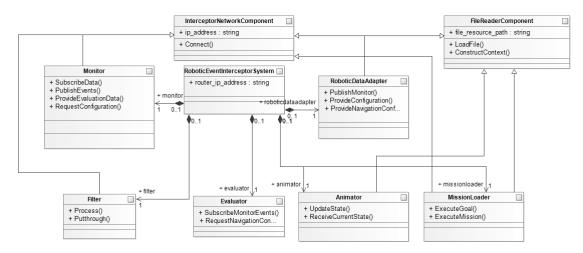
Figure 24. Component setup of the system
