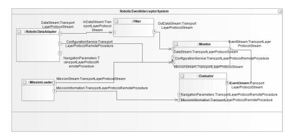
Figure 25. Network interconnection of components
