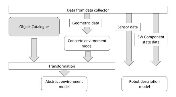
Figure 19. Runtime model reconstruction based on incoming data
