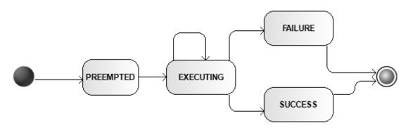
Figure 22. Simplified state machine of action execution
