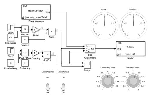
Figure 27. Dashboard to teleoperate ROS-based robot in simple scenarios
