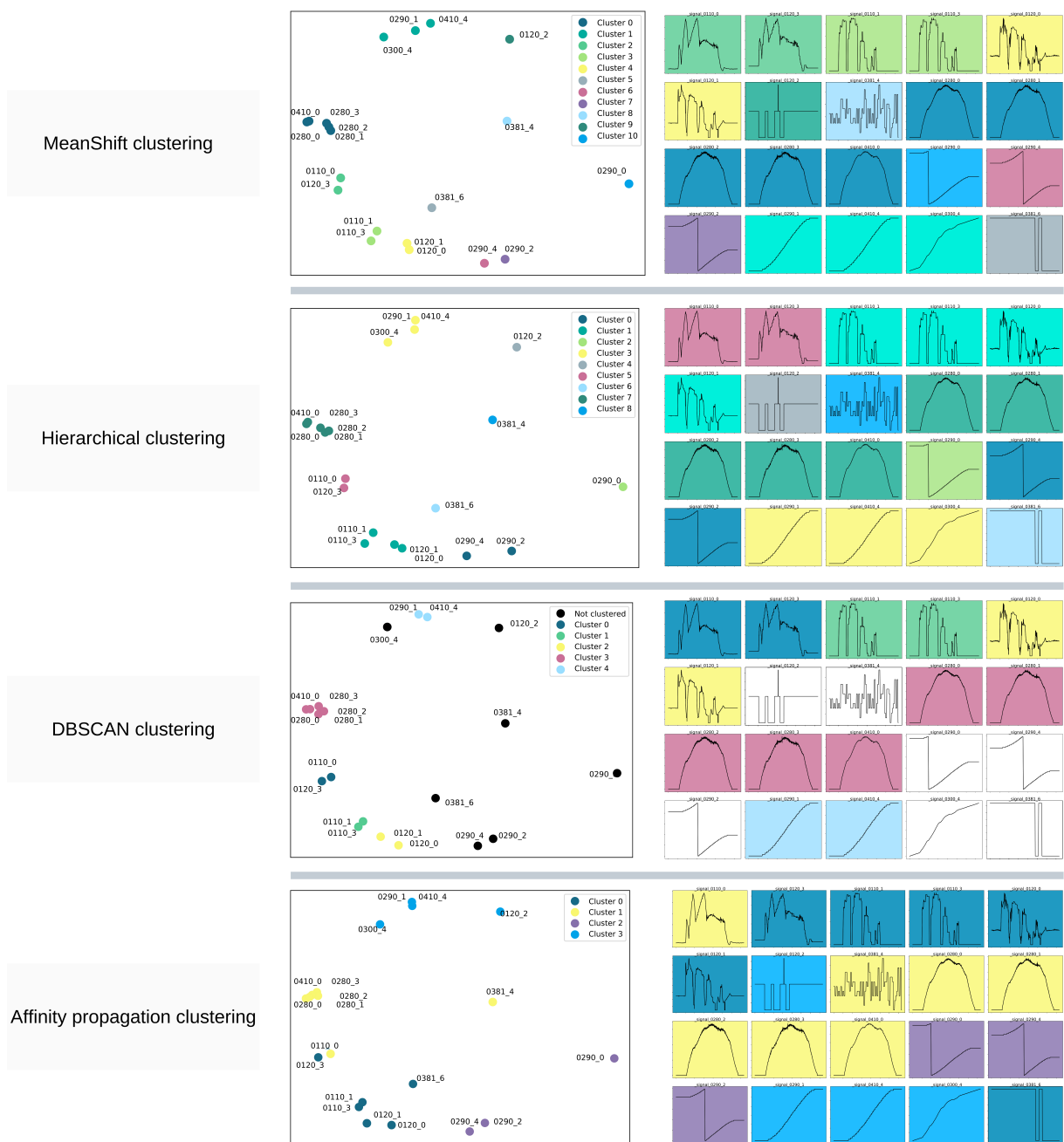
Figure 5.2: Comparing signal groups produced by different clustering techniques, with different correlation metrics. From top to bottom, the result for 1) MeanShift clustering with Spearman correlation, 2) Hierarchical clustering with Pearson correlation, 3) DBSCAN clustering with Kendall correlation and finally 4) Affinity propagation clustering with Spearman correlation can be seen. First column indicates the name of the chosen pair of clustering and correlation method, second column shows a 2D representation of the clustering, while the first column shows each signal, with the same background color for each signal in a group.
