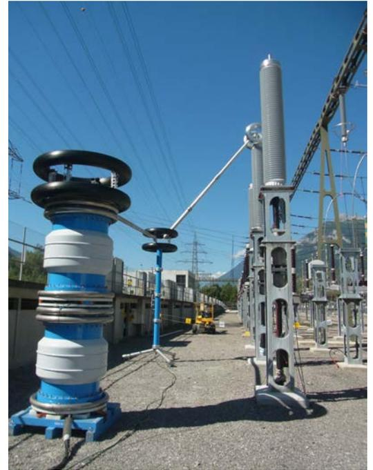
Figure 3-4: The on-site measurement setup with the HV test installation
