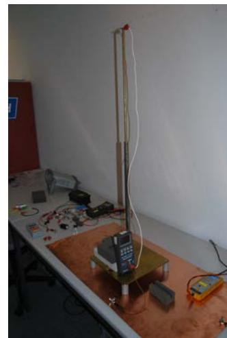
Figure 4-16: Measurement setup for the  $C_{\text{Core-Ground}}$  measurement
