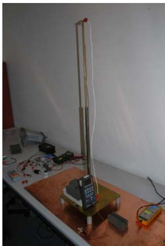
Figure 4-15: Calibration setup for the  $C_{\text{Core-Ground}}$  measurement
