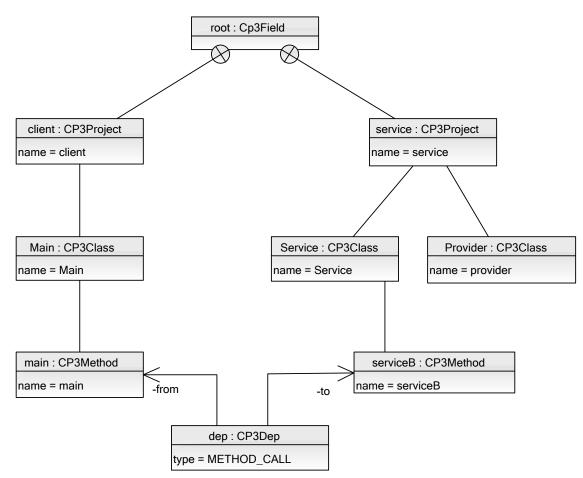
Figure 4.15: Elements of the compacted instance model
