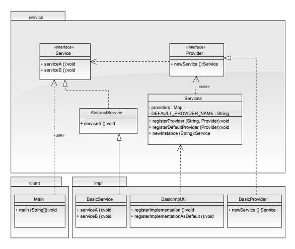
Figure 3.3: Structure of Service Provider Framework design pattern
