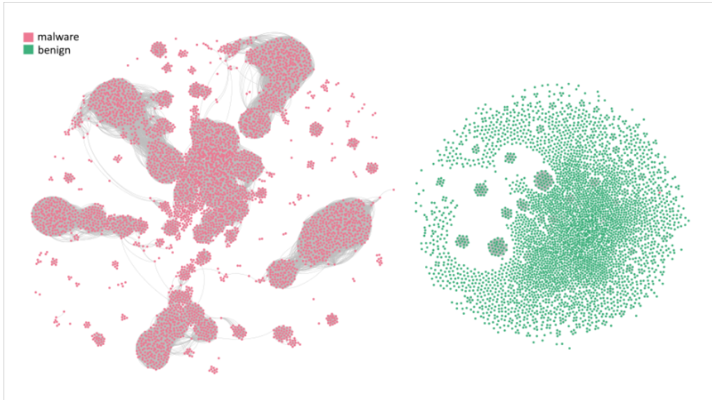
Figure 2.1: Illustration of a similarity graph of a set of binaries. Vertices represent the binaries and two vertices are connected with an edge if the corresponding files are similar according to some similarity measure. In this figure, two files are considered to be similar, if their TLSH difference score is below the threshold 40, where TLSH is a locality sensitive hash function and TLSH difference is a TLSH-based dissimilarity metric. Malware binaries are represented by red nodes and benign binaries are represented by green nodes. As it can be seen, there is no similarity between malware and benign files and the malware similarity graph is strongly clustered.
