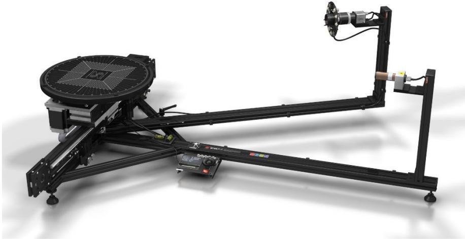
Figure 3: The 3D scanner with the laser, the camera, the two motors, the controller and the turntable
