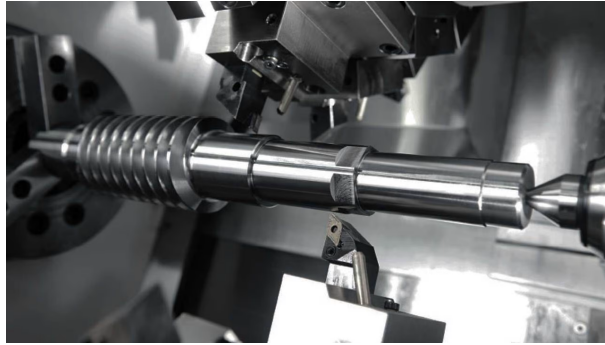
Figure 2.2: A complex workpiece machined by turning, with pre-existing milled surfaces in a hexagonal pattern
