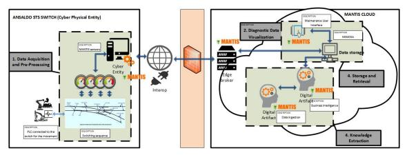
Figure 3.7: Instantiation of the MANTIS architecture for railway switches
