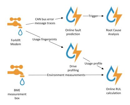
Figure 3.6: Overview on stream processing data flow for RUL and online fault prediction engines
