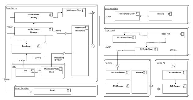
Figure 3.4: Instantiation of MANTIS for industrial press machines1
