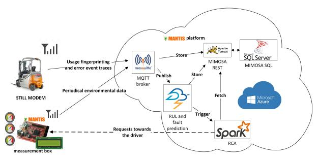
Figure 3.5: Instantiation of MANTIS for forklifts
