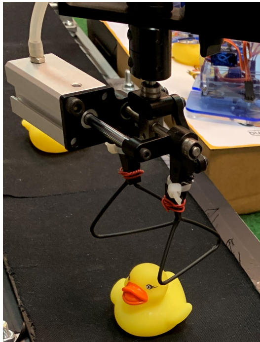
Figure 7.3: The custom clamp that allows the robot to grab rubber ducks
