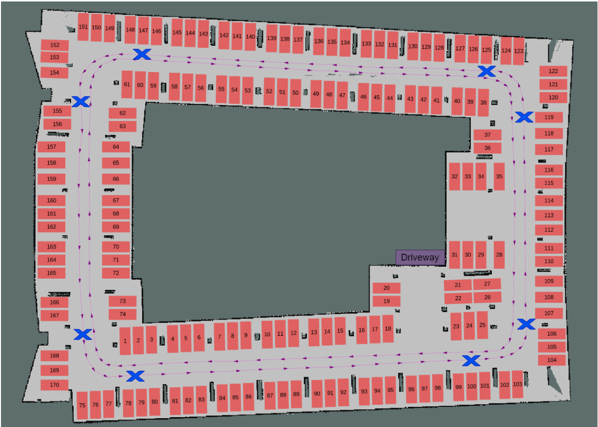
Figure 5.2: The parking garage with the parking spaces. The purple box indicates the driveway from the upper level while the blue crosses denote the eight navigation goals. The small arrows constitute the TrackGraph.
