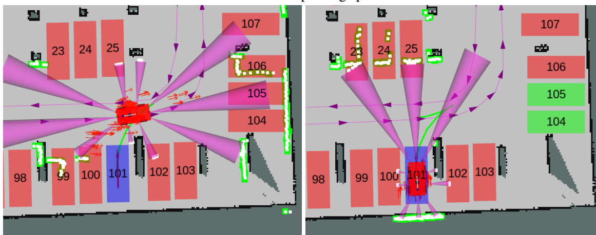
(c) If there is a preferred parking space, path planner will be changed from Hybrid A* to RTR+CCRS (d) Car parked to the preferred parking space and other parking spaces were successfully detected (spot 104 and 105) as well
