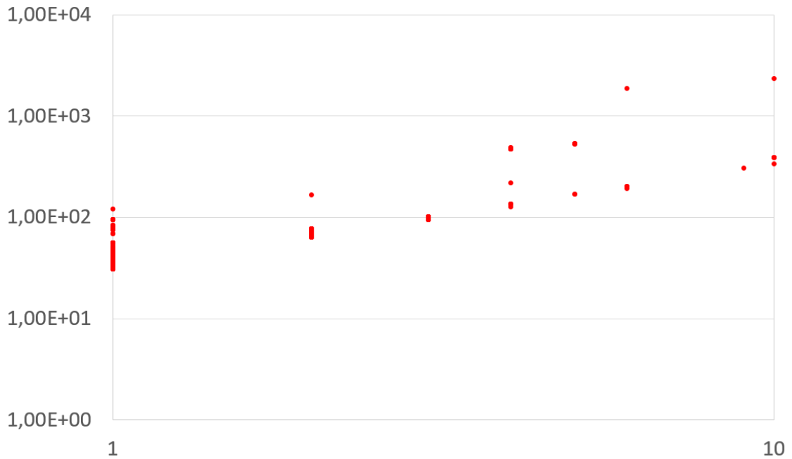
Figure 3.4: Downlink traffic flow distribution of APN "A2" (x axis: number of packets, y axis: Size of flows [Byte])
