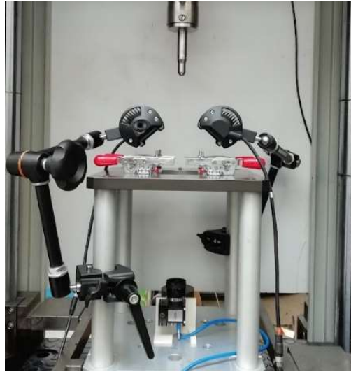
Fig. 14. Static Indentation test setup with camera and backlights.
