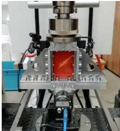
Fig. 15. Compression after indentation test setup with camera and backlight.
