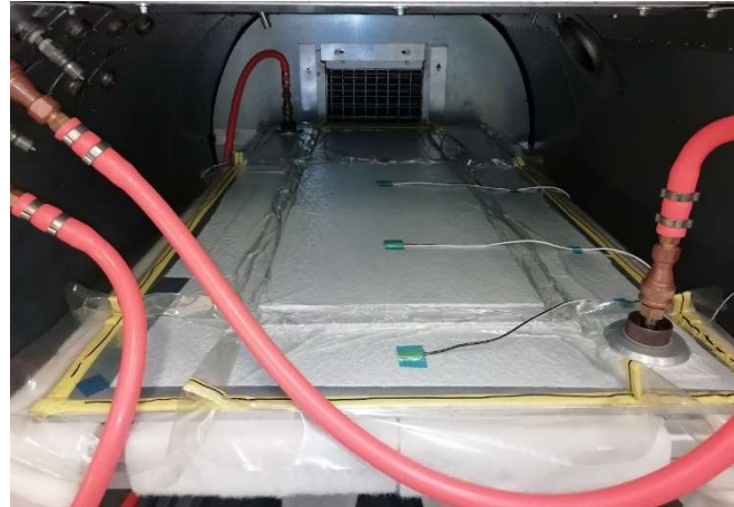
Fig. 13. The tool plate with the laminates in the autoclave.
