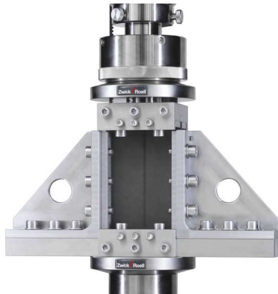
Fig. 10. Zwick Roell compression after impact support fixture [17].
