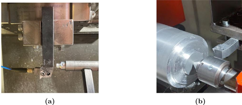
**Figure 4.8:** (a) Initial setup with the tool directly positioned on the Kistler, (b) new setup with a compliant tool holder inserted in between the tool and the Kistler
