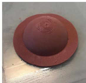
**Figure 4.10:** The final silicone shell
