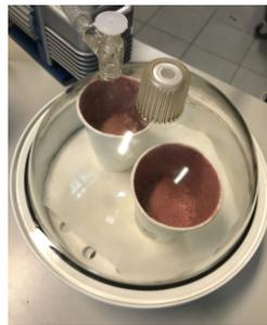
**Figure 4.6:** Degassing the silicone in the vaccuum chamber
