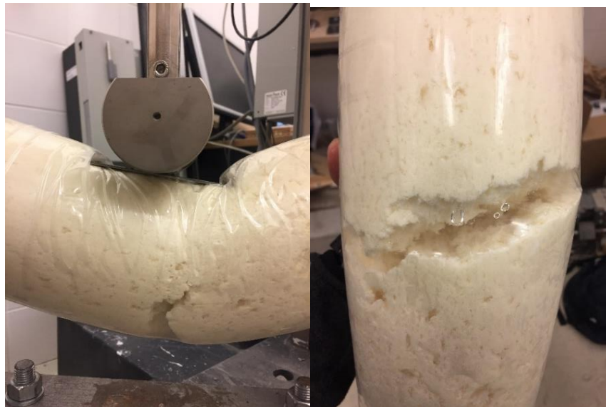
Failure of one of the beams at its midpoint
