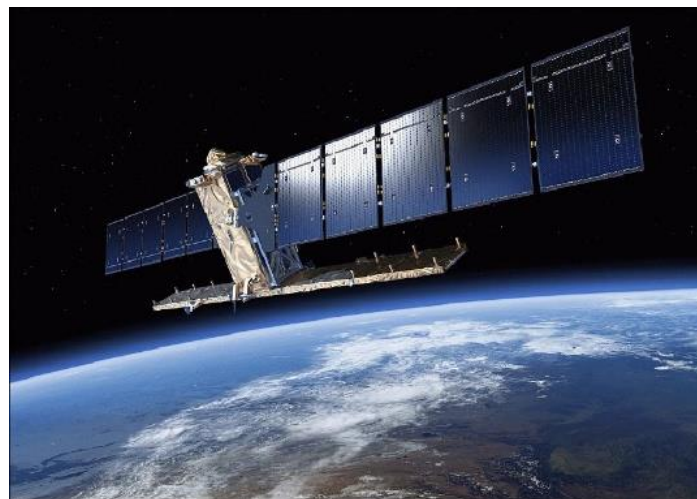
View of the deployed Sentinel-1 spacecraft with large deployable solar panels (image credit: ESA, TAS-1)
