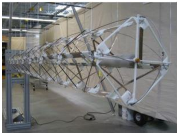
K-truss Boom with Quadrifilar Helical Antenna Under Test
