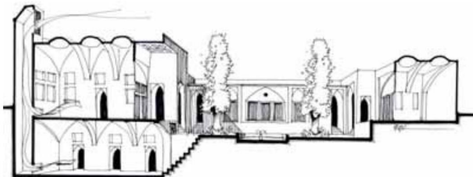
Figure 19. Schematic section of a “house for four seasons” with a one sided wind tower above the summer living quarter (Source: Ali Tavakoli Dinani)
