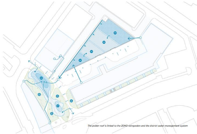
Figure 21/The polder roof water management sequence. It can handle stormwater storage and reuse in a controlled way by using smart applications
