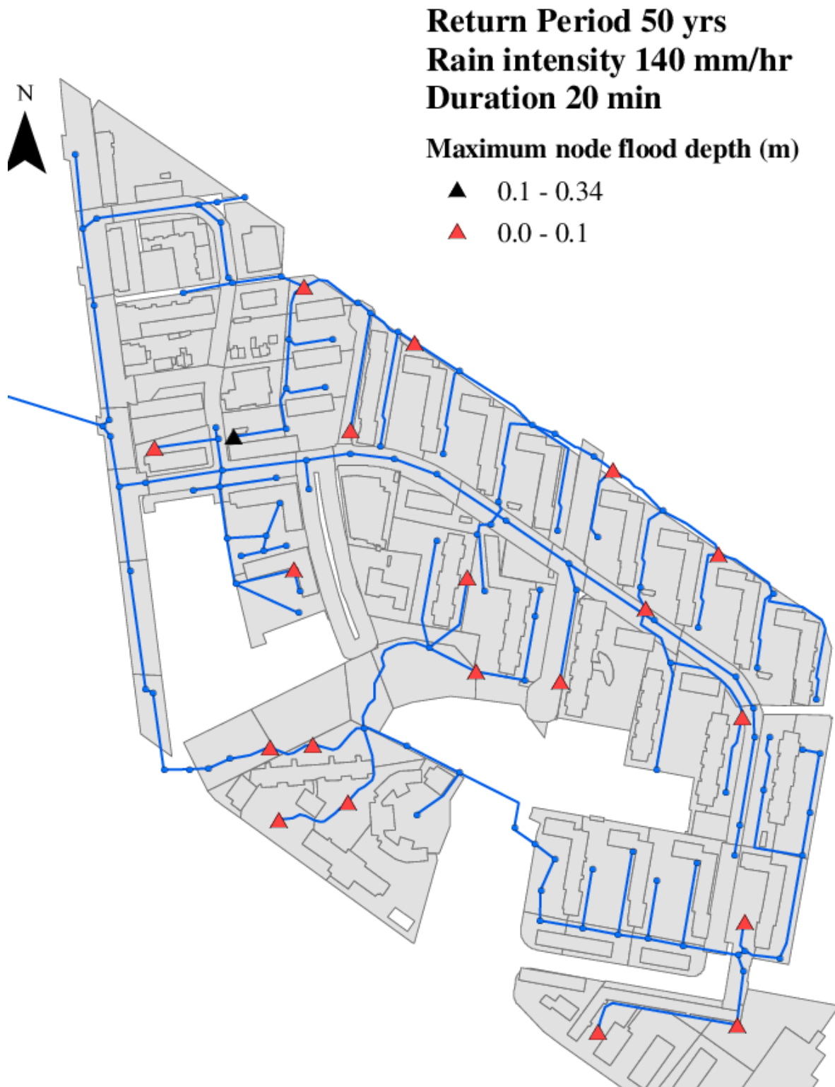
Figure 27/Maximum node flooding in the open stormwater system caused by the 140 mm/hr intensity rainfall for the duration of 20 minutes.
