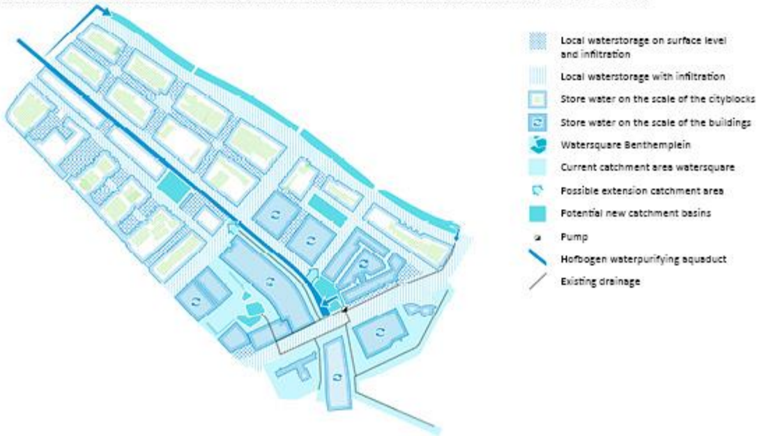
Figure 22/map diagram with legend for managing local water system in ZOHO district
