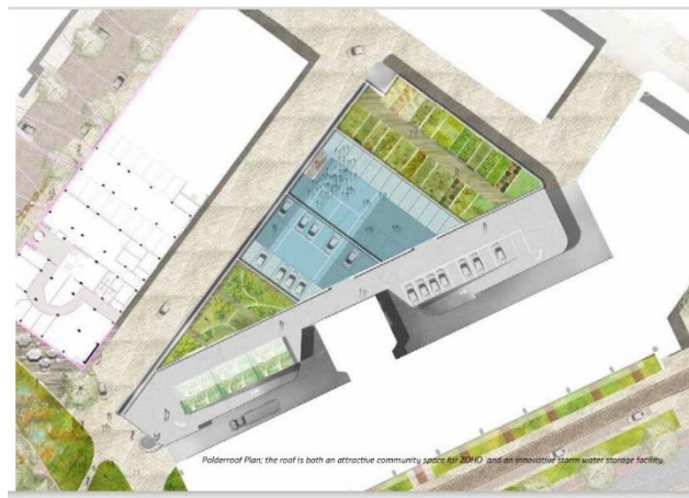
Figure 20/Polderroof Plan; the roof is both an attractive community space for ZOHO and an innovative storm water storage facility
