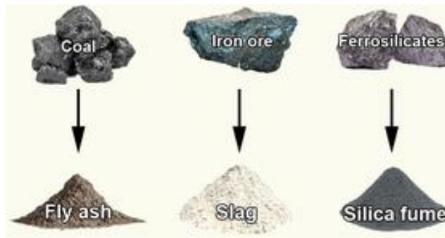
**Figure 3:** Common examples of SCMs made of byproducts (waste materials) (EMS-CP, 2020)
