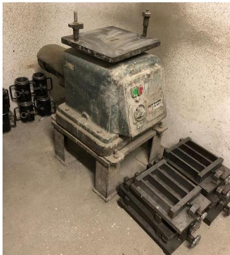
**Figure 11:** Compaction table
