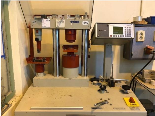
**Figure 14:** Flexural tensile and compression device
