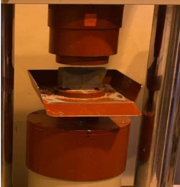
**Figure 16:** Compressive strength machine
