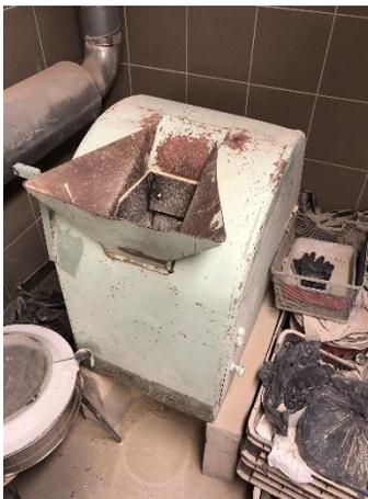
**Figure 6:** Jaw crusher
