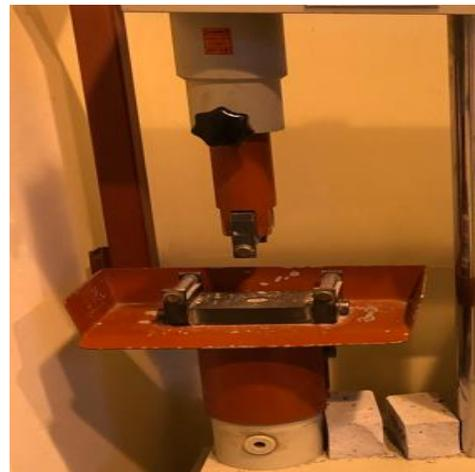
**Figure 15:** Flexural tensile device
