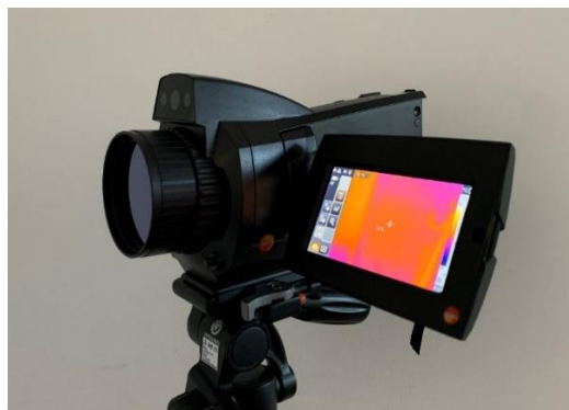
Figure 3. testo 885-2 used in the experiment
