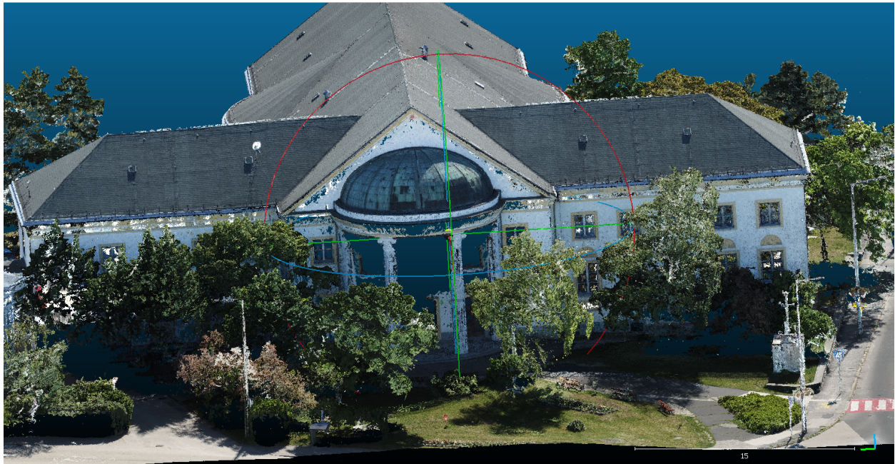
Figure 16. The western facade of the building as seen in the DJI Phantom 4 Pro point cloud
