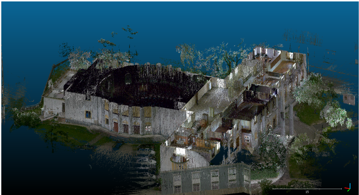
Figure 21. Section of the first floor of the building as seen in the Leica BLK2GO point cloud(RGB)
