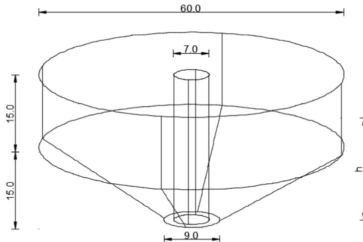
Figure 2 - Geometry of the model [cm]
