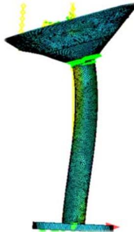
*Figure 1 - Resonance of a water tower - numerical model*
