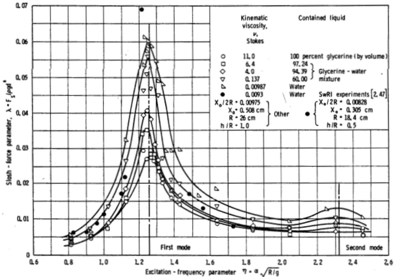
Figure 3 - NASA result - conical tank, viscosity is changed
