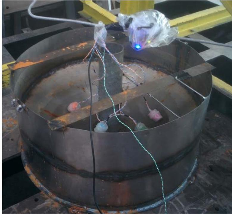
*Figure 9 - Accelerometers*
