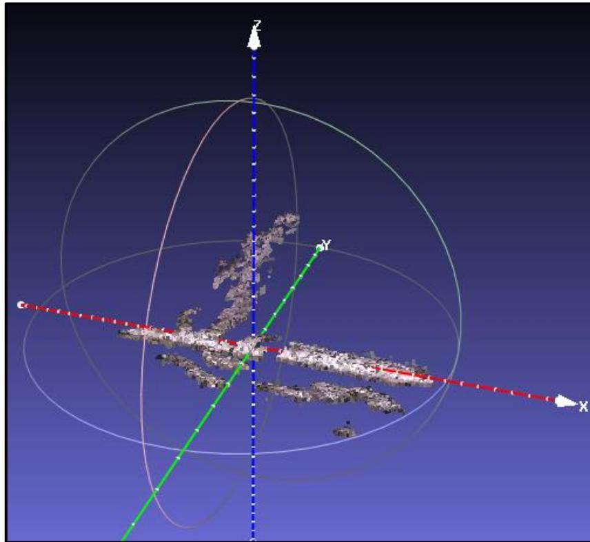
*Figure 15. Cleaned and axis-fixed 3D mesh of the groyne in Meshlab*
