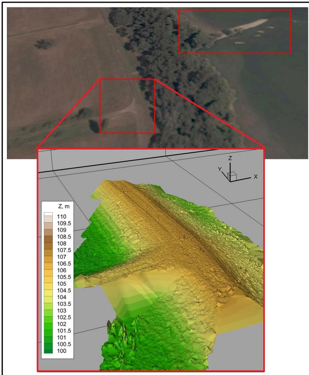
**Figure 12.** Cleaned and georeferenced surface of the dyke visualized in Tecplot
