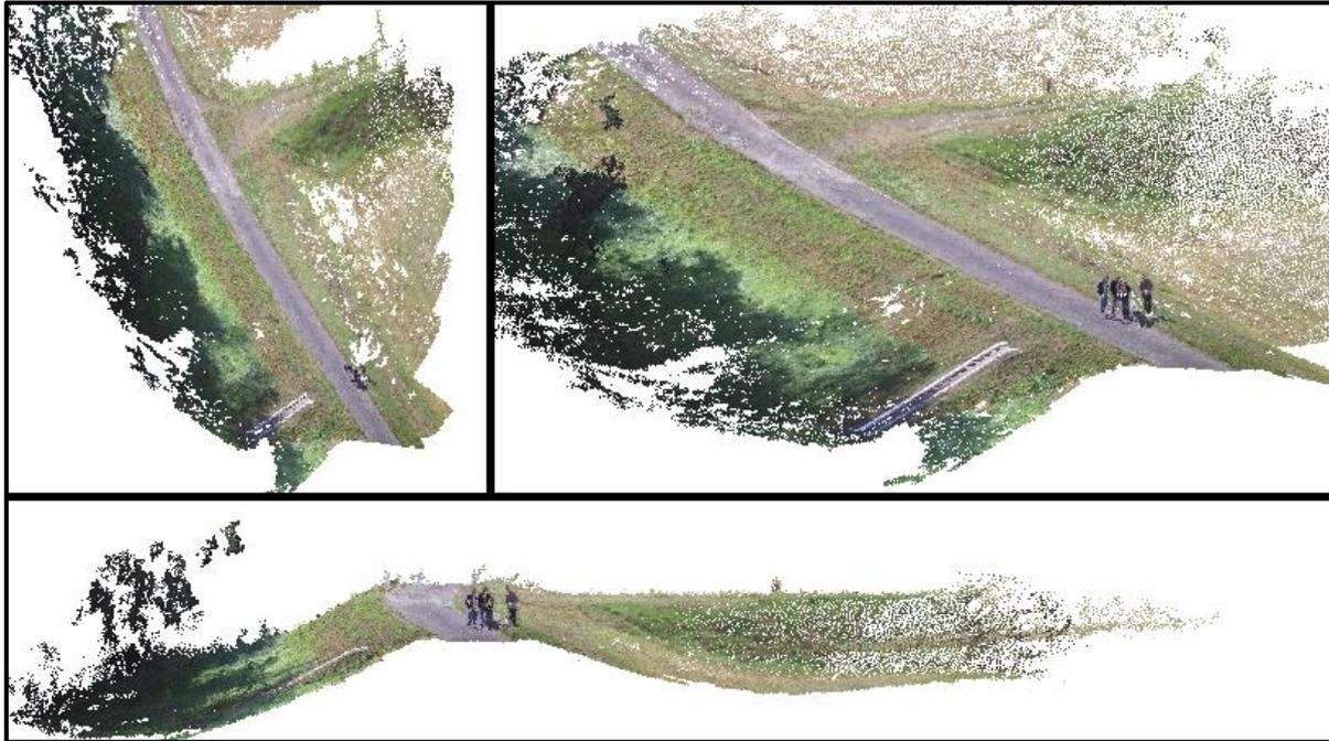
**Figure 10.** Raw 3D dense point cloud of the dyke from different views in VisualSFM
