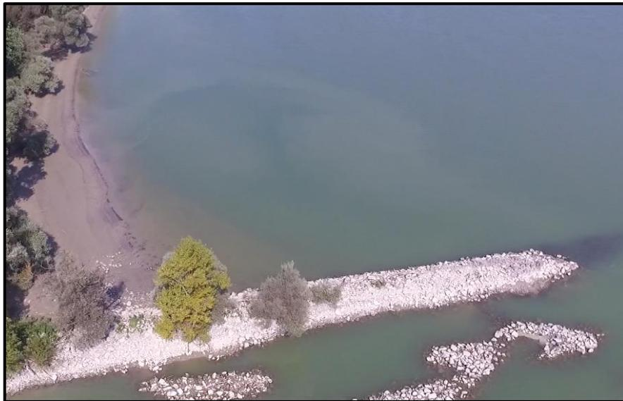
**Figure 38.** *Sediment resuspension patterns seen from the UAV*
