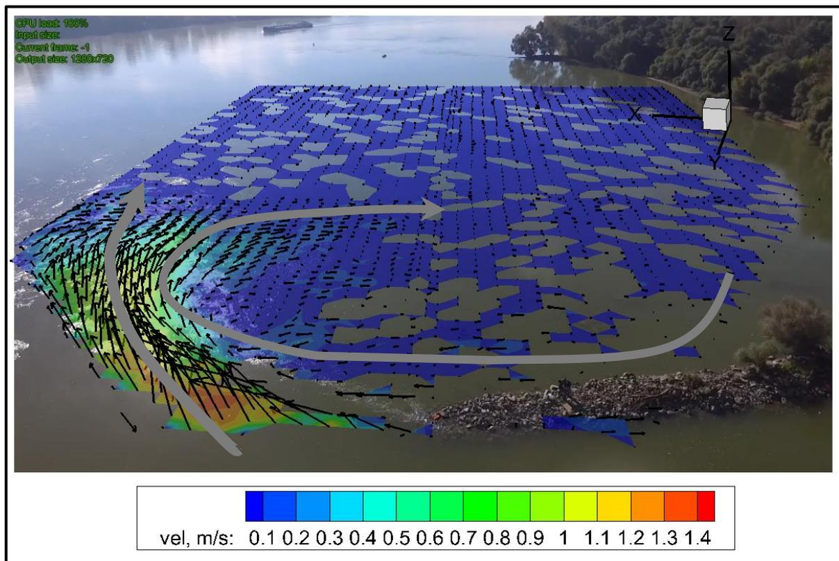
**Figure 21.** Surface velocity distribution near the groynes from UAV-based LSPIV measurements (perspective view)
