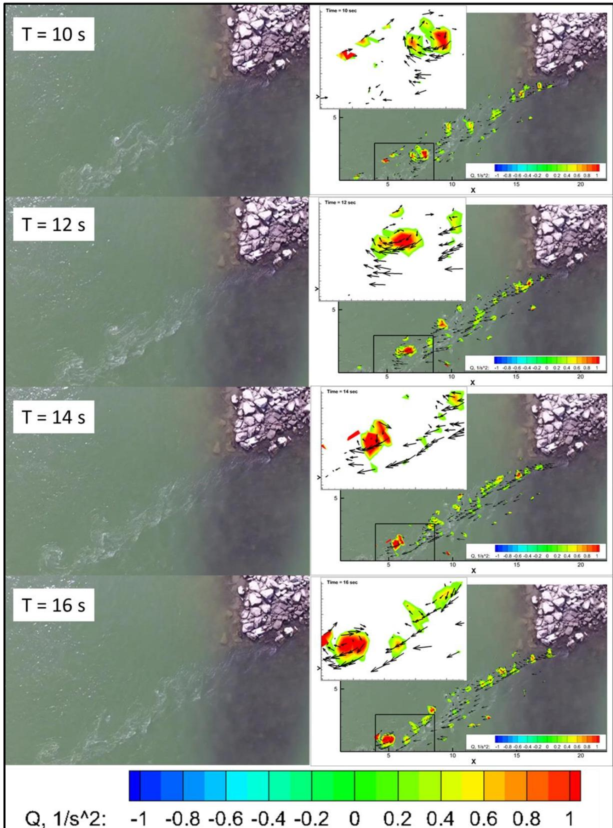
**Figure 26.** Q distribution near the groyne from LSPIV analysis
