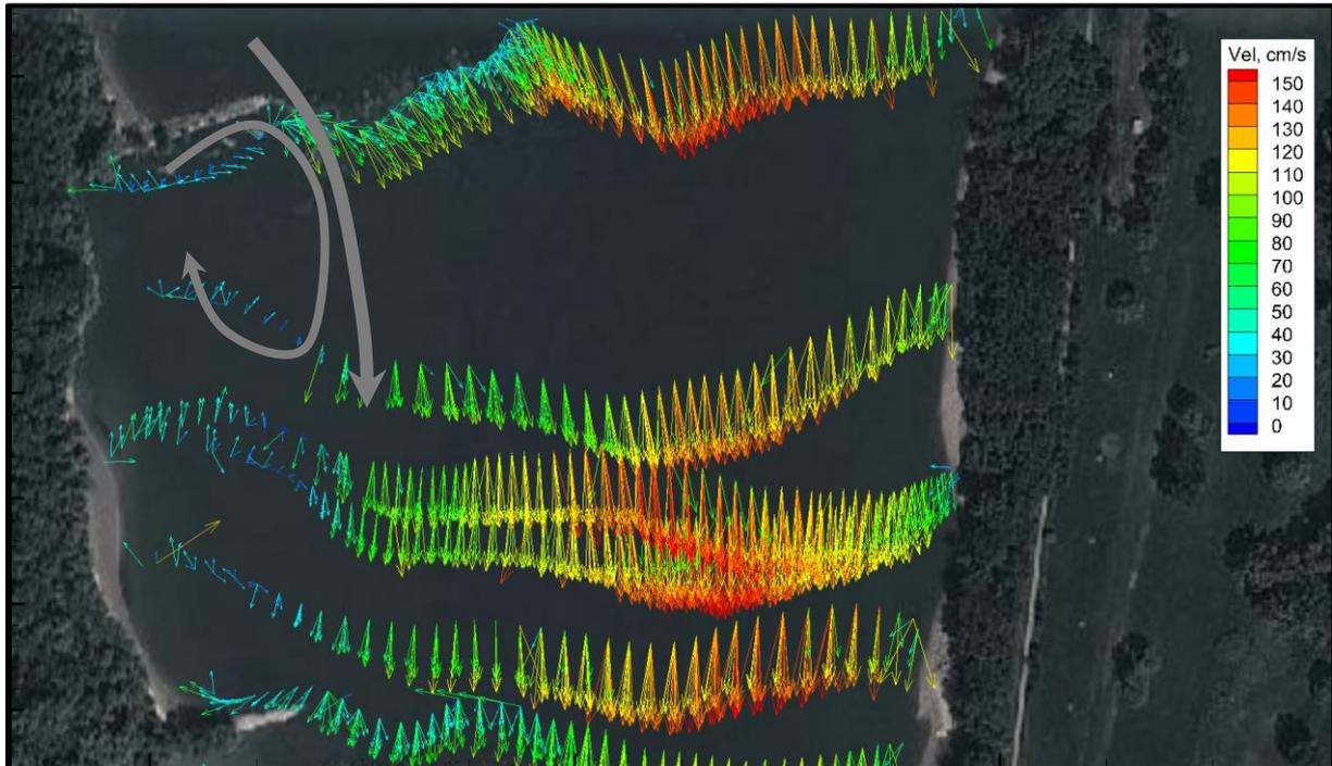
**Figure 22.** Surface velocity vectors from moving boat ADCP measurements (Fleit, 2013)
