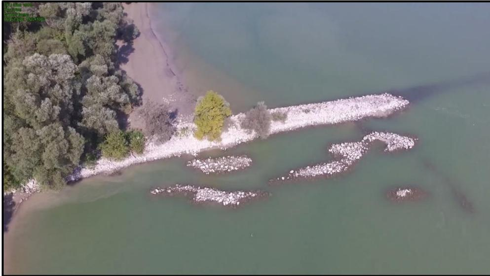
**Figure 13.** Raw image of the groyne from the UAV
