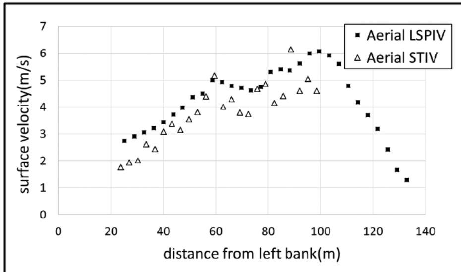
**Figure 33.** Comparison of stream wise velocity distributions. By two methods at a cross section upstream from a bridge. (Fujita et al., 2016)
