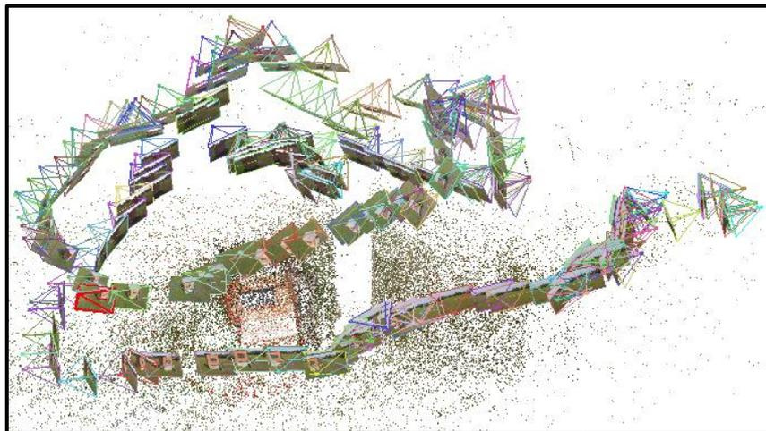
**Figure 8.** Calculated camera positions around the point cloud of the radial well in VisualSFM
