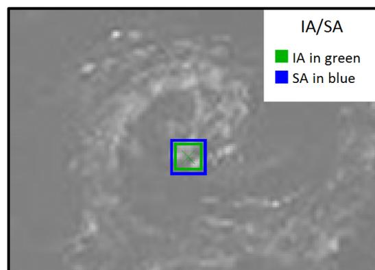
**Figure 24.** IA/SA settings in eddy-scale LSPIV analysis
