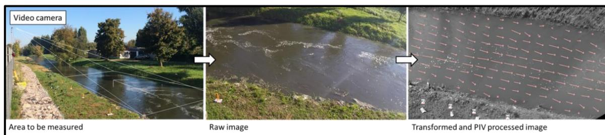
**Figure 15.** LSPIV measurement sequence
