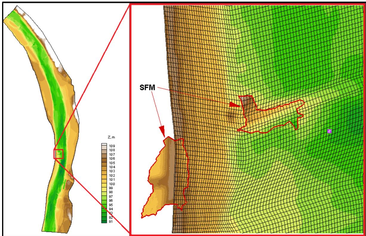
*Figure 17. SFM-made 3D objects added to DTM in SMS software*
