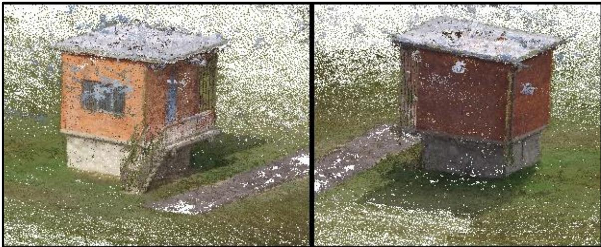
**Figure 7.** Raw 3D dense point cloud of the radial well from different views in VisualSFM
