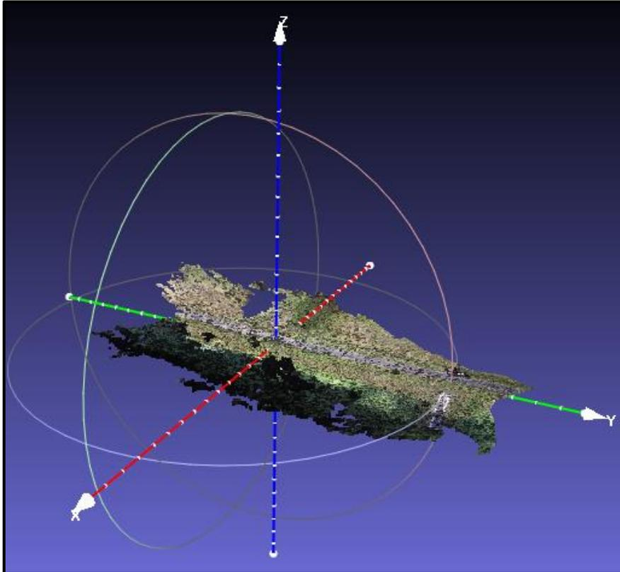
**Figure 11.** Cleaned and axis-fixed 3D mesh of the dyke in Meshlab
