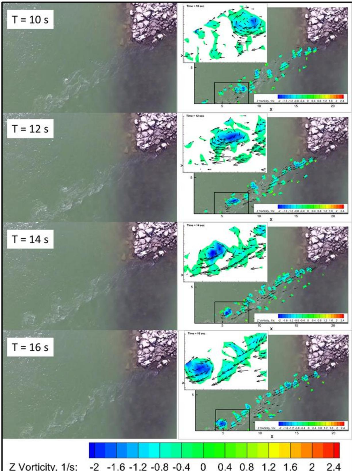
Figure 25. Z Vorticity distribution near the groyne from LSPIV analysis
