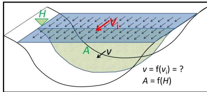
**Figure 18.** Index velocity in the surface velocity field
