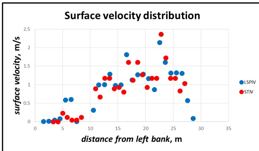
Figure 37. Velocity distributions with LSPIV and STIV methods
