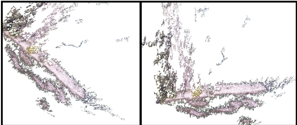
**Figure 14.** Raw 3D dense point cloud of the groyne from different perspectives in *VisualSFM*
