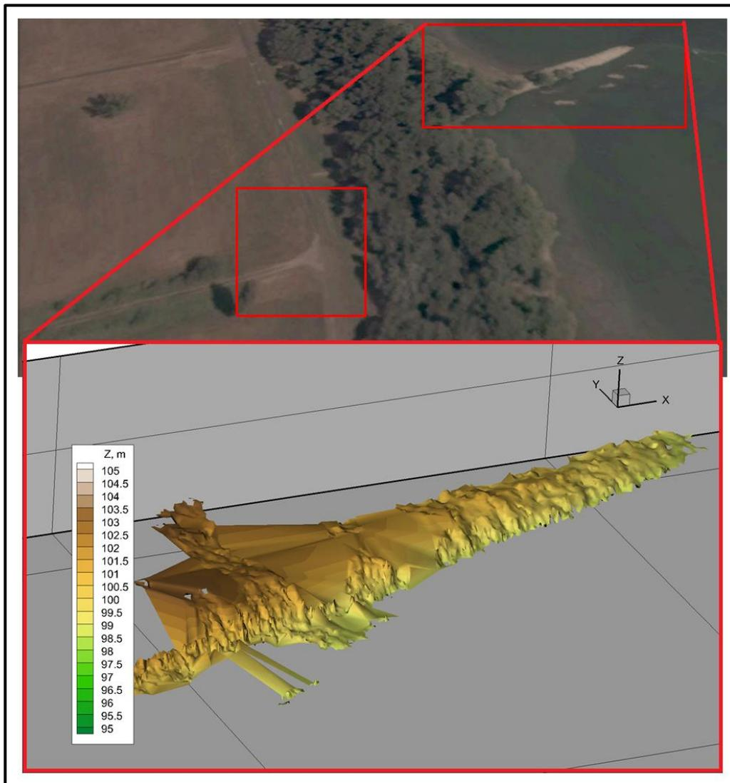
**Figure 16.** Cleaned and georeferenced surface of the groyne in Tecplot
