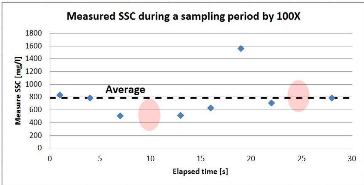
Figure 33 Measured SSC sequence for a sampling period
