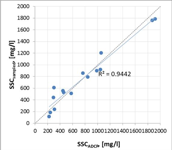
Figure 27 Calibration of the ADCP (Campaign K01)
