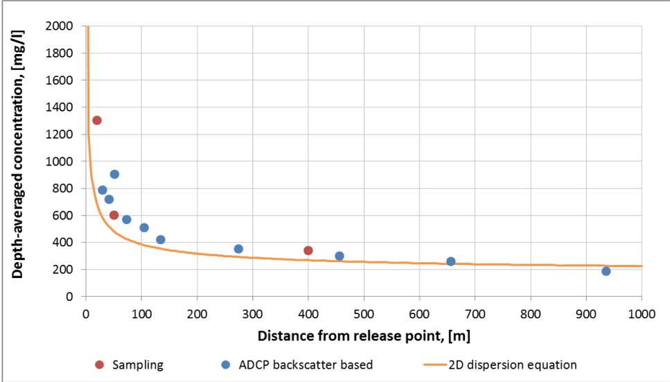
Figure 30 Longitudinal profile of the SSC (Campaign K01)
