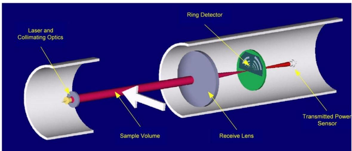
Figure 1 The working method of the LISST (Sequia Scientific Inc.)
