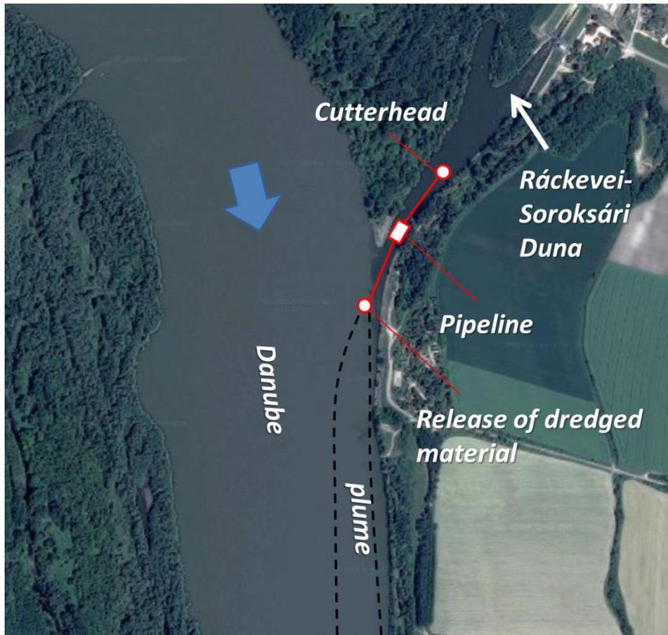
Figure 25 Dredging site at the downstream end of the side-branch of the Danube (Downstream 'Tass' lock)
