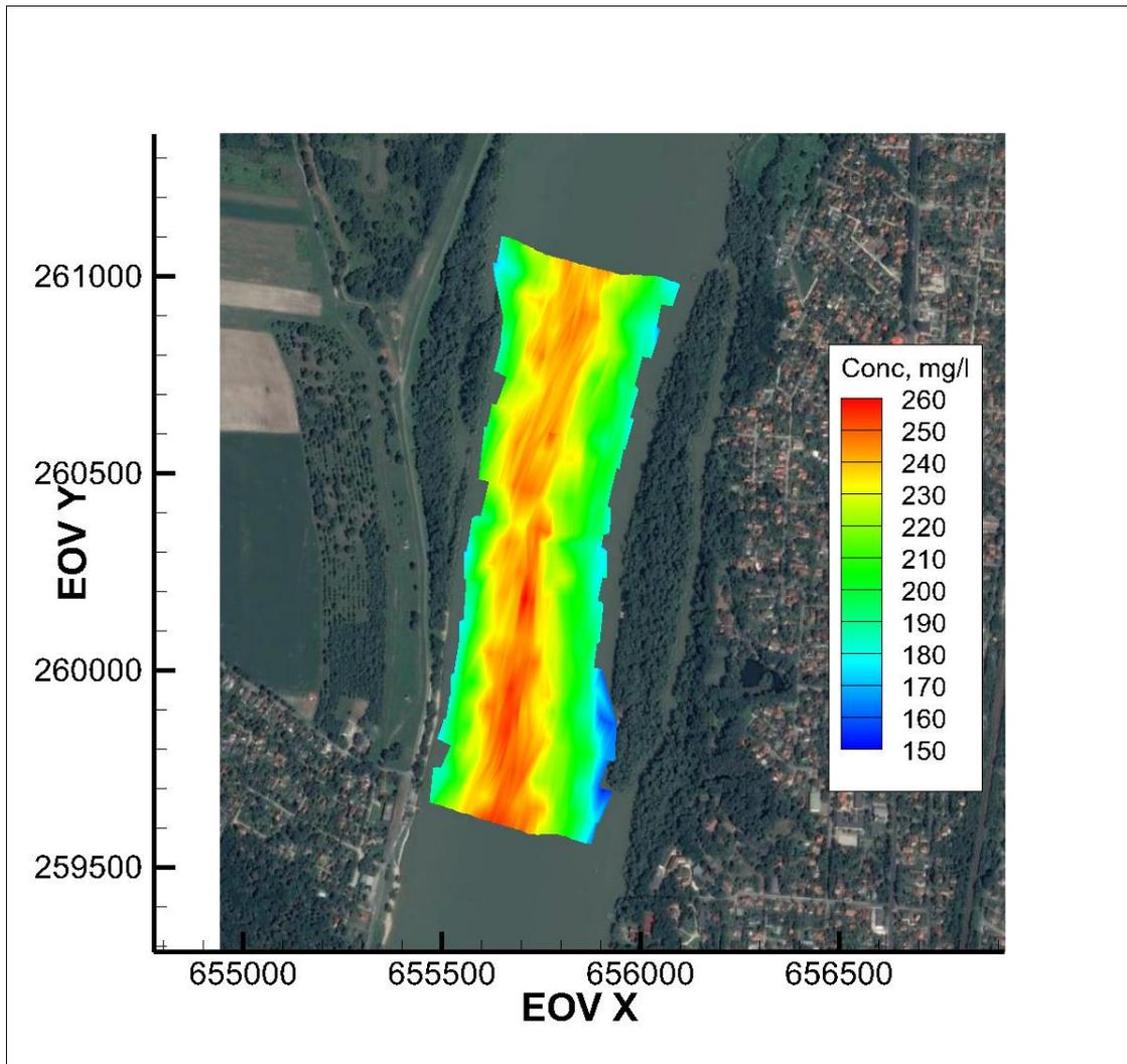
Figure 23 SSC field according to the OBS data
