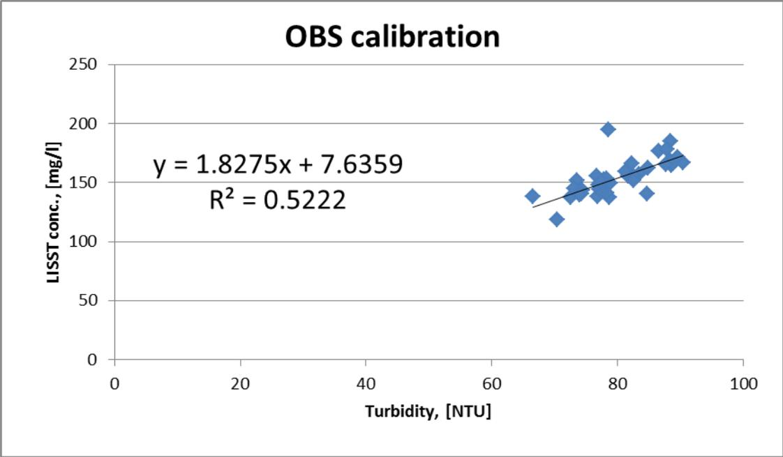
Figure 21 Calibration of the OBS according to the results from Transect A
