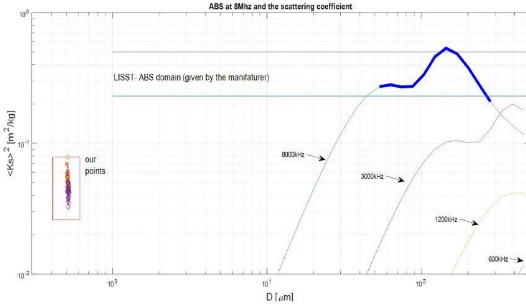
Figure 17 Calibration values for the LISST-ABS (Conevski et al, 2016)
