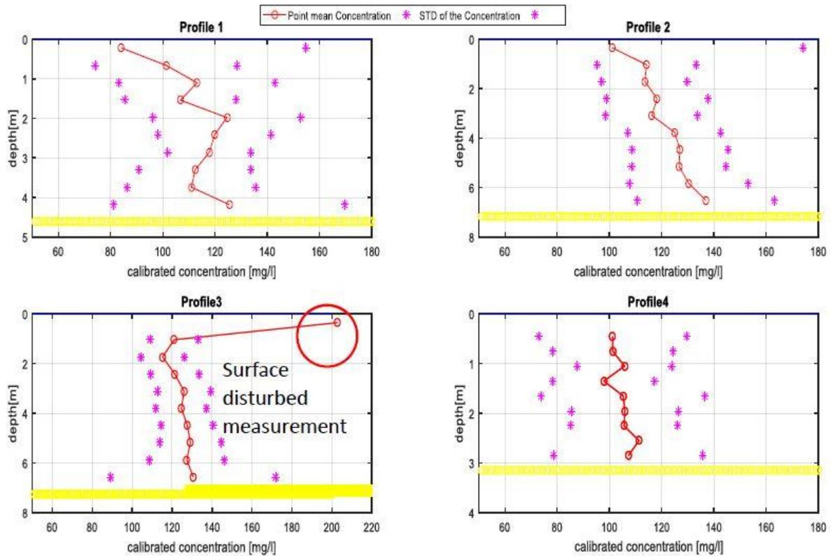
Figure 19 SSC profiles by the ABS (Conevski et al, 2016) at Transect A
