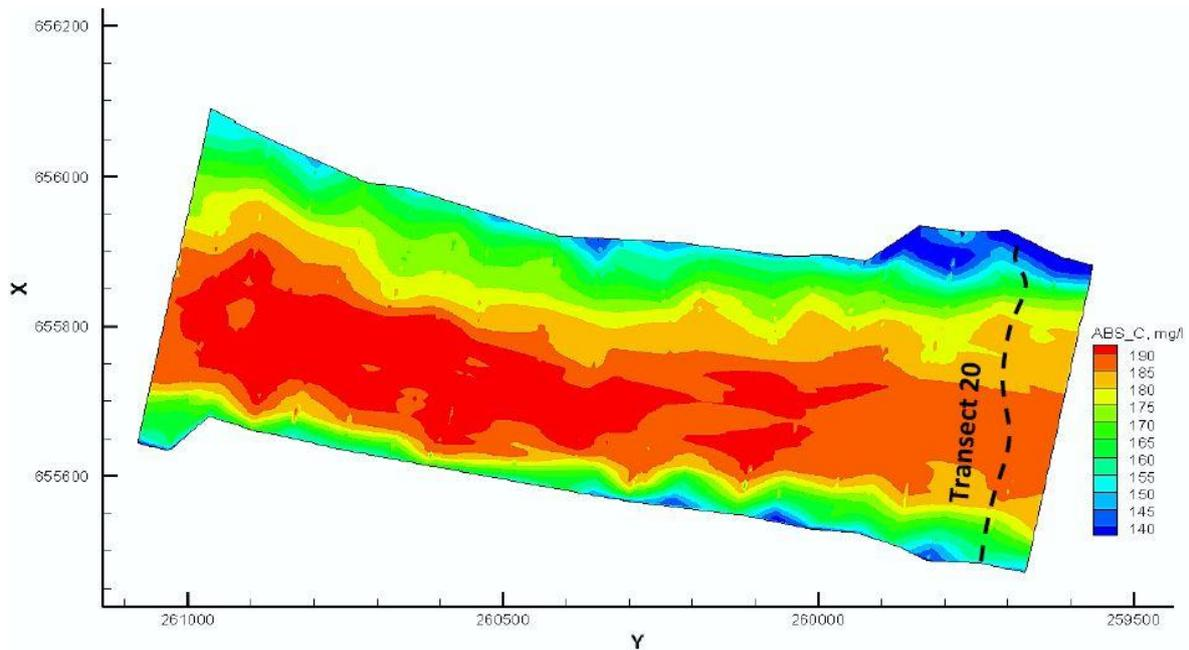
Figure 20 SSC map according to the ABS results (Conevski et al, 2016)
