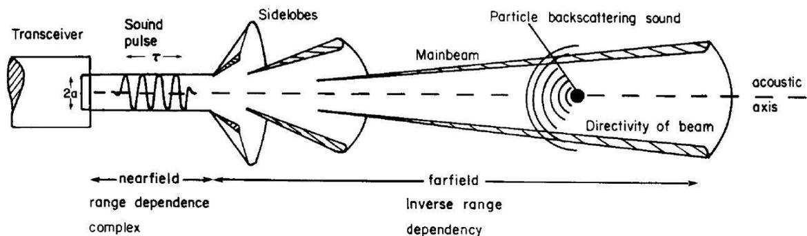
Figure 6 Scheme of the working principle of acoustic devices (Thorne et al, 1990)
