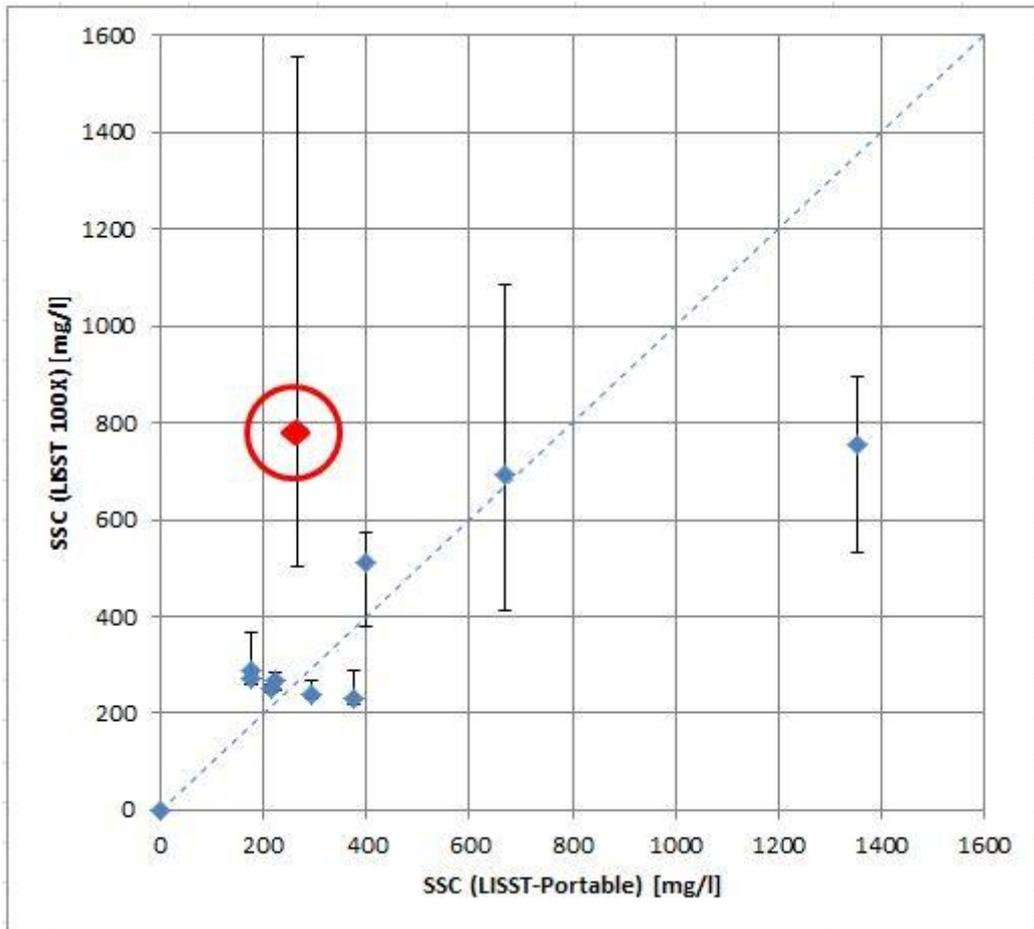
Figure 32 LISST100X values against LISST-Portable results
