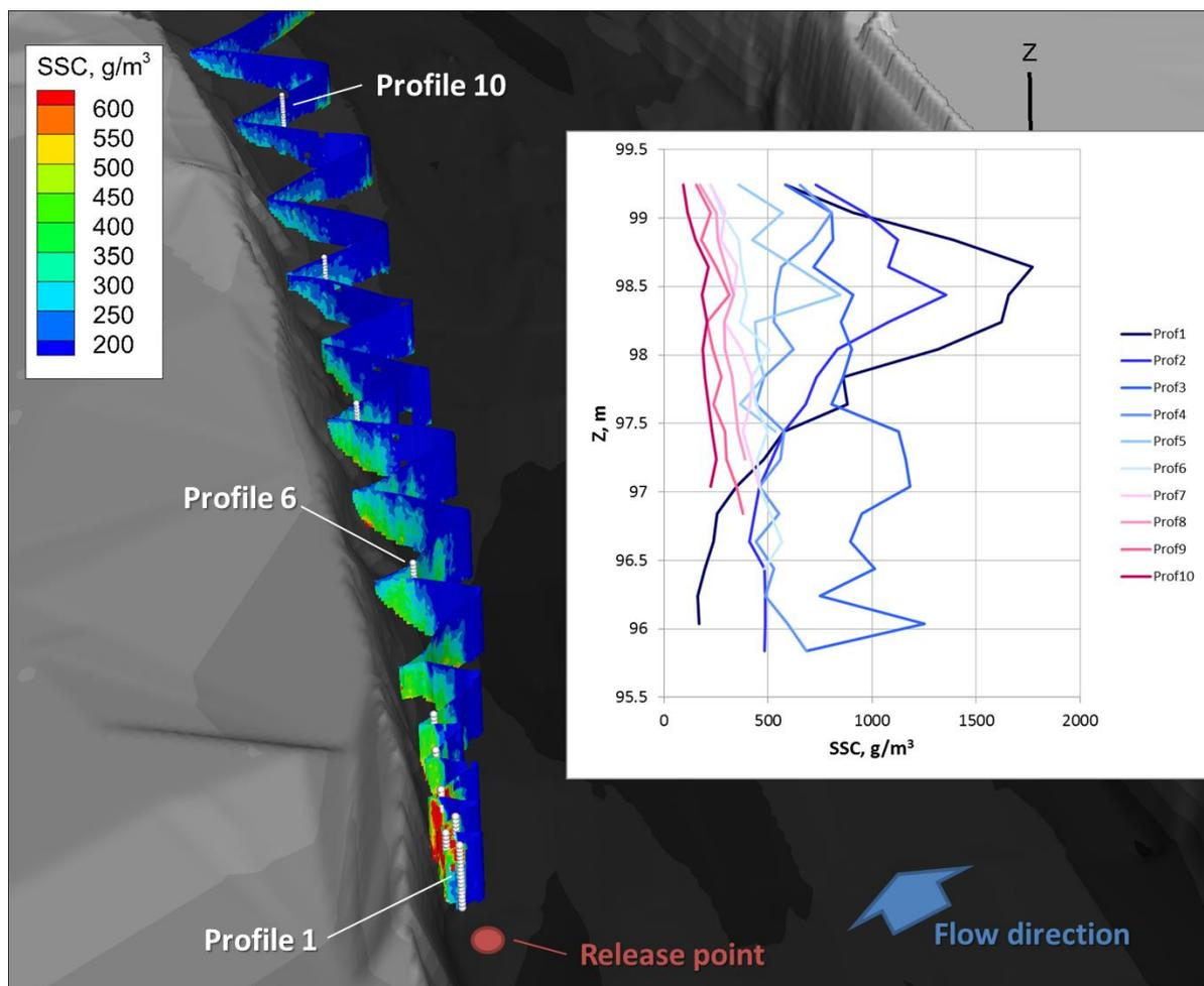
Figure 29 Shape of the plume and SSC profiles by ADCP from campaign K01
