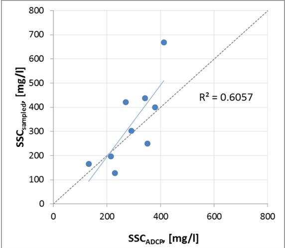
Figure 28 Calibration of the ADCP (Campaign T02)
