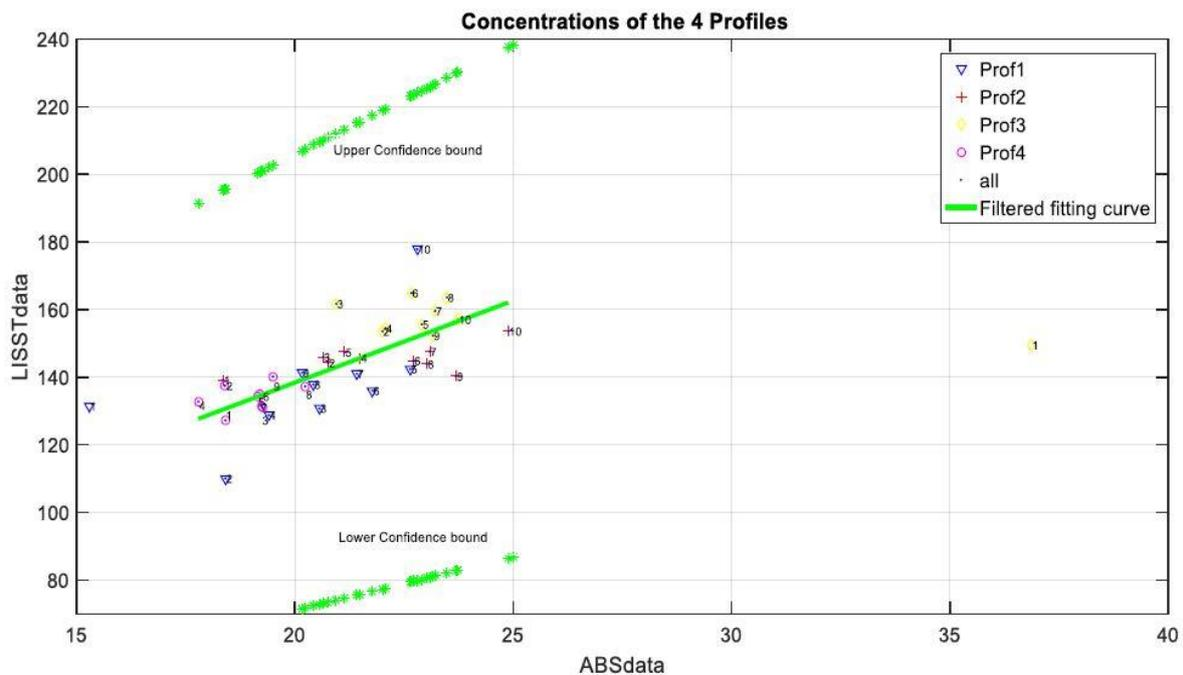
Figure 18 Calibration of the ABS (Conevski et al, 2016) according to the measurements at Transect A
