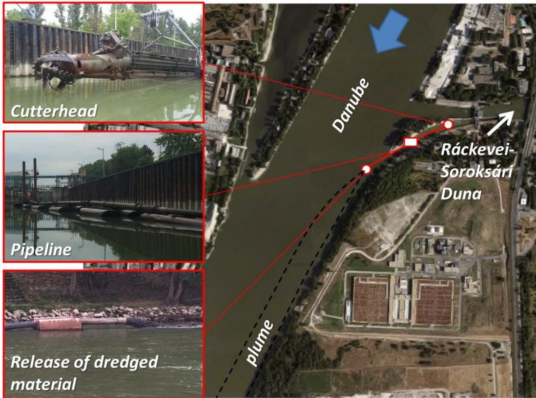
Figure 24 Dredging site at the upstream end of the side-branch of the Danube (Upstream 'Kvassay' lock)
