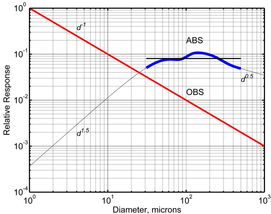
Figure 7 Comparison between OBS and ABS responses (Agrawal et al, 2016)
