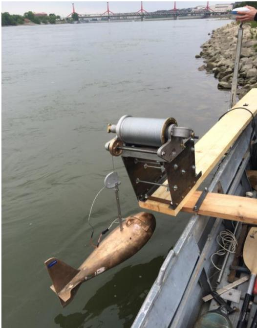
Figure 10 US P-61-A1 sampler and its setup
