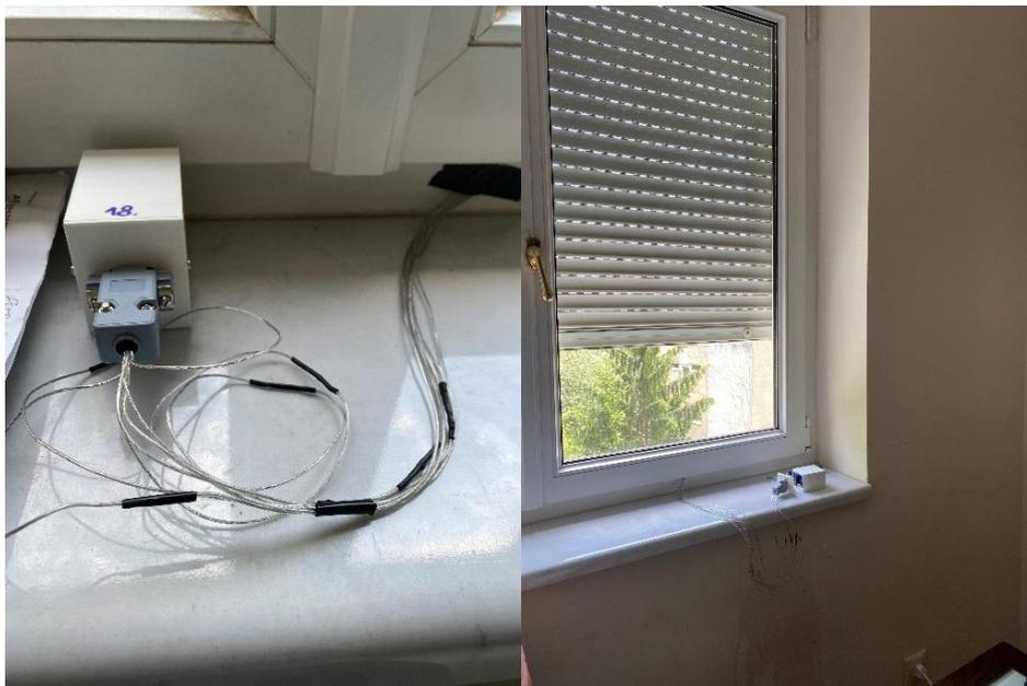
*Figure 7 - Window monitoring in-situ assembled device. Photo: Dóra Szagri*
