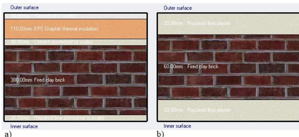
Figure 3 - Layers of walls (a - external, b - internal)
