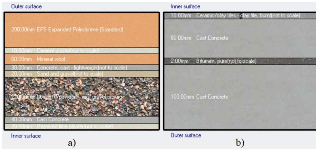
Figure 4 - Layers of flat roof (a) and ground slab (b)
