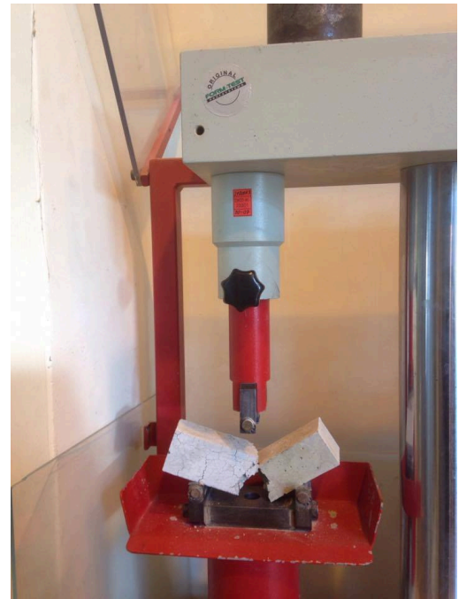
Figure 9. Bending test after loading
