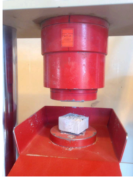
Figure 10. Compressive strength test
