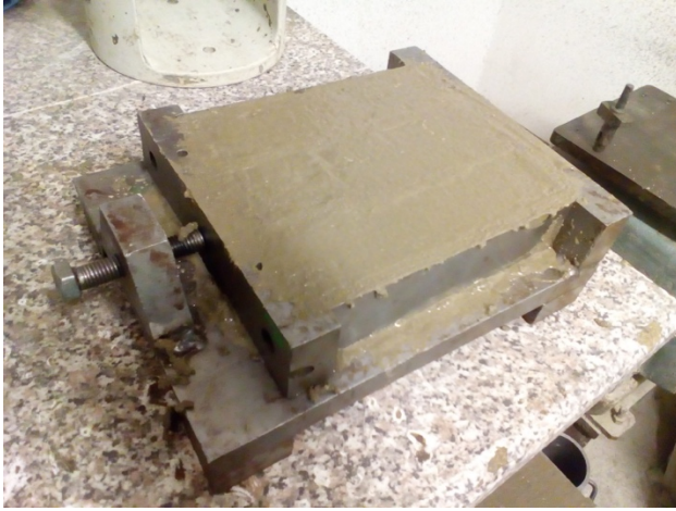
Figure 5. Fresh mortar in the mould
