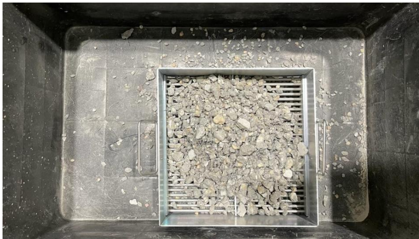
Figure 5.9.7 – Filtering of free steel fibres from C2D RCA
