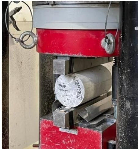
Figure 4.2.1 – Installation of splitting tensile strength test
