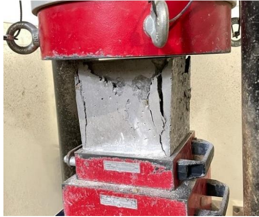
Figure 5.1.9 – Compressive strength test, specimen failure
