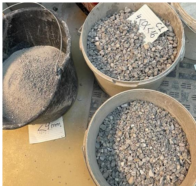
Figure 5.9.1 – Crushed and sieved aggregates C1: 0/4 (left), 4/16 (right)
