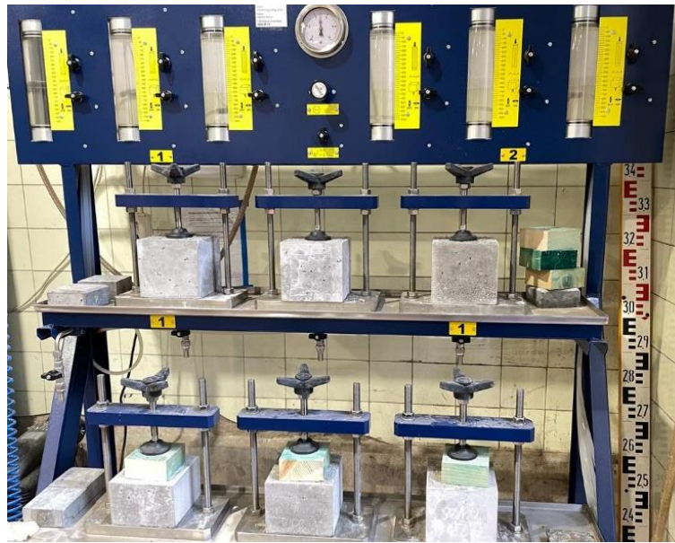
Figure 4.5.1 – The water permeability test setup.
