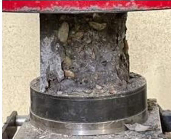
Figure 5.7.1 – Freeze-thaw specimen failure under compressive stress
