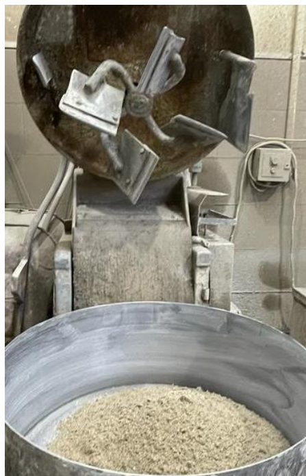
Figure 3.3.1 – Concrete mixing machine
