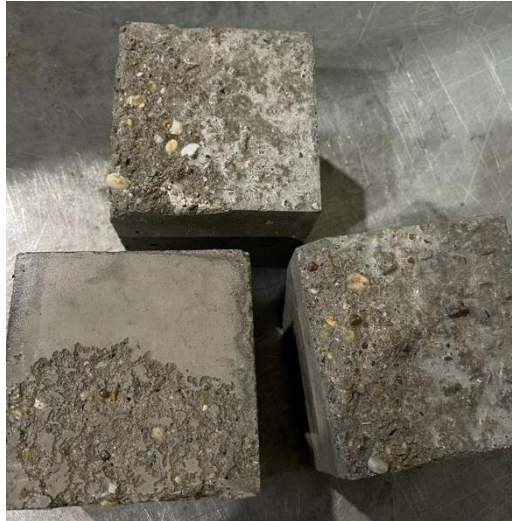
Figure 5.8.5 –Surface deterioration C1, Generation II
