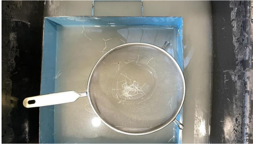
Figure 5.9.6 – Filtering of free PP fibres from C2M RCA
