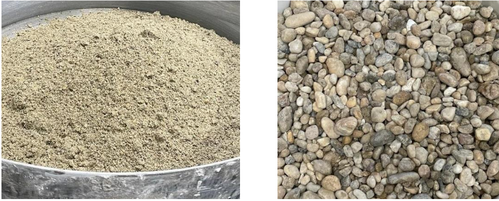
Figure 3.2.1 – NA:0/4 (left), 8/16 (right) fractions
