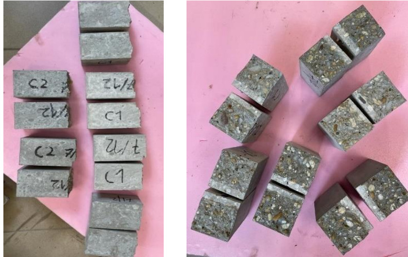
Figure 5.3.13 – CMOD test specimens after failure
