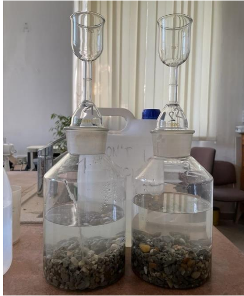
Figure 5.9.8 – RCA in pycnometer – apparent density test
