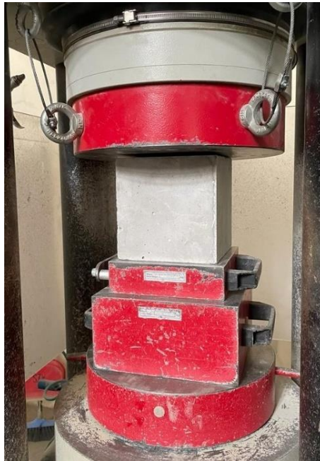
Figure 4.1.1 – Installation of compressive strength test
