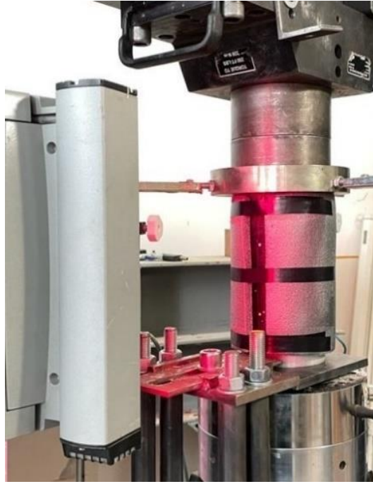
Figure 4.6.1 – Testing for stress-strain behaviour
