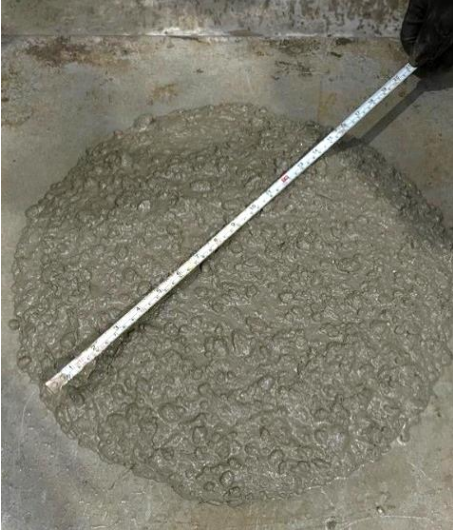
Figure 3.3.2 – Flow table test
