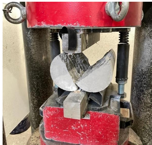
Figure 5.2.1 – Splitting tensile test, specimen after failure.
